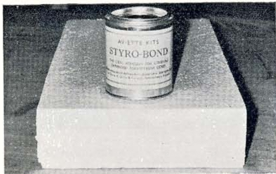
A block of Expanded Polystyrene, as used by Aviette Kits to prepare hot-wire cut wing cores and the special adhesive they advise known as "Styro-Bond".
