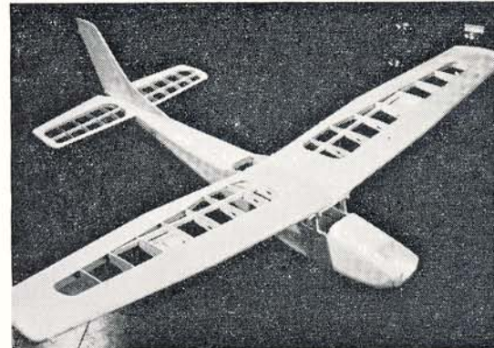
The uncovered airframe of the 62" span Cessna Skylane, built from a standard kit. Spacious fuselage will take a variety of Radio gear. Right: The Airfix He 177-5A is an extremely finely detailed model with the usual moving surfaces, turrets, propellers, etc. that are virtually standard on the larger models.
