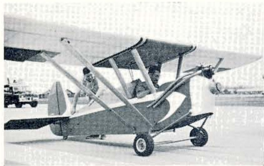
F/Lt Ray Lawrence made this ultra-light for a Triumph motorcycle engine while with 66 Squadron at Kuching in Sarawak. Thus it became the first aircraft to be made in that Country. Test flights were successful; but a posting back to Singapore meant that it had to be dismantled. Subsequently it became the Fokker DR1 seen on the cover. Needless to say, Ray is an aeromodeller.
