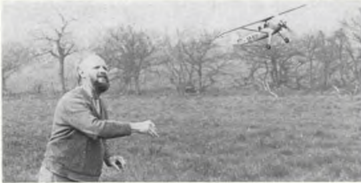
Away she goes! The little Kania does what she likes best . . . flying. This is an ideal prototype for a 'first' scale model - nice high wing layout with ample tail surfaces makes for a stable machine.
