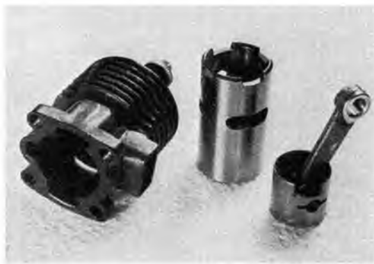
KMD features one-piece diecast alloy cylinder jacket, encasing Schnuerle ported liner.
