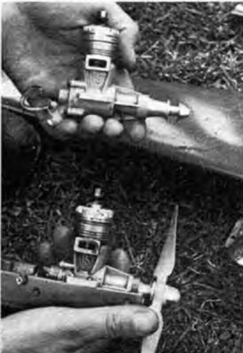
A couple of diesel-converted K & B 15's. The motor at bottom recorded fastest heat and final in FAI team race, using Boughton 7 x 7in. and Graham Howard's 'South African' glass fibre preparations.
