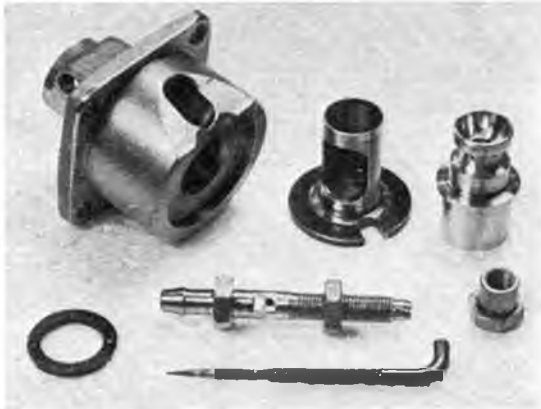
KMD Induction unit has drum type rotary valve and a multi jet carburettor.
