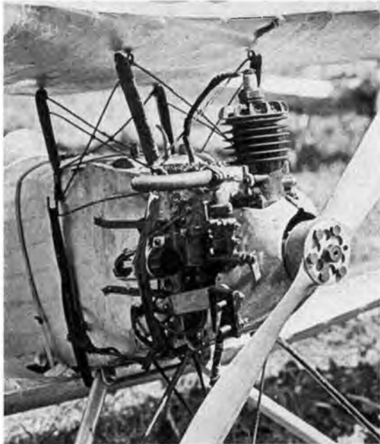
The 28cc Wall, reduced to 56oz from its original much heavier model boat installation was almost half the total weight of Capt Bowden's 'Kanga' record holder. Ignition was kept handy on outside of fuselage!
