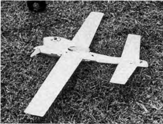
An FAI speed model flown at NZ Nationals, powered by a Westland 15 and fitted with an experimental mini pipe.
