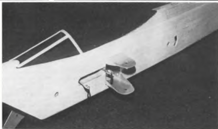
Top left is Brian (Mr Stuka) Dyke's latest 'biggie', conforming to the current trend of twin fins and tricycle undercarriage. To the right is shown one of the detachable wing panels - and just take a look at that beautiful structure. A work of art. Below that is a close-up of the fuselage, revealing the aluminium stubs onto which the wing panel is bolted. Note too the holes for the locating dowels at both leading and trailing edge positions. At left is the Super Tigre 46 mounted on Marco Beschizza's MM 'Centrefire' kit. The engine mount (supplied in kit) bolts to a plywood former bonded to the ABS fuselage. Note horizontal joint lines of fuselage - easily disguised by the paint trim.
