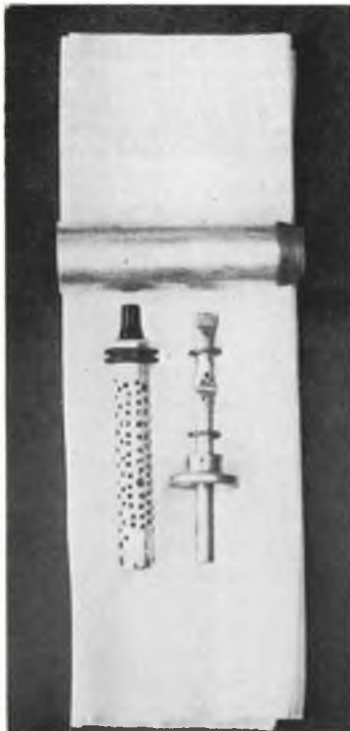
Below are the basic components of the add-on unit, namely the Ronson gas refill, piece of aluminium tube (old TV aerial), plus Pentel felt pen. At bottom is the completed, assembled unit. The 'modified' components are shown at left, together with the Kleenex tissue wadding.
