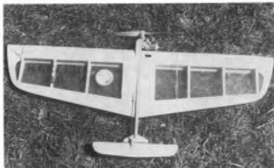
Ira Keeler's WAM Class A combat design shows current US approach (models flown to FAI rules but with up to 3.5cc engines). Single boom tail mount and large sheeted leading edge still popular - but giving way to foam.
