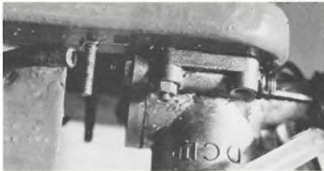
Tail heavy models will not fly and may need the engine moving forwards to correct balance. Use original front bolt through rear lug hole and fit extra bolts at front. Move fuel tank forward also to give correct feed.
