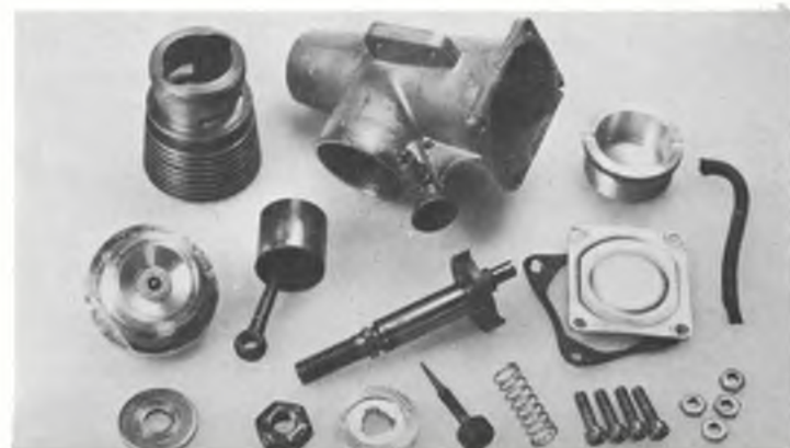
The Fox 09 engine of 1959 referred to by one of our readers. A very easy to operate beginner's engine that could be bought for less than £2.50 in the UK. We could do with some of these today! Spread of components at right reveals that main casting included small fuel tank as well as crankcase. Intake was via piston controlled cylinder port. Engine could be beam or radially mounted.
