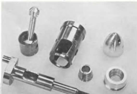
Most notable feature revealed by CSTKAM parts is its large parallelogram shaped angled transfer ports which give Schnuerle type gas flow. Other parts include neat diecast crankcase, ground all-over crankshaft finish and peripheral jet carburettor.
