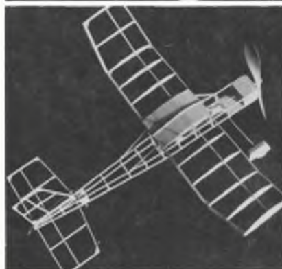
Above: Peck Polymers Prairie Bird designed for the US Embryo Endurance rules, should fly well by virtue of light construction. Below: C/L goodies from the left: 100cc syringe, alum. tube, rubber tube and pacifiers for fuel tanks, circular bellcrank and housing, 1\frac{1}{2} in racing wheel, bushed steel Fox bellcranks large and small, 1oz glass cloth, Aldridge Magnum handle with Fox C/L connections, small, medium and large.
