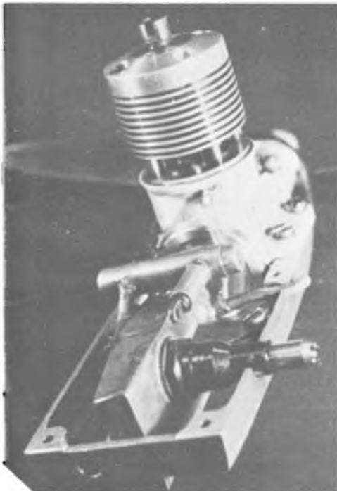
Above: Oliver Cub installed in pan showing exhaust primer pipe running from overflow T junction through circular flange on crankcase. Right top: Inside of engine cowling shows venturi intake, shut-off reset button and pan fixing holes. Middle: Air inlet and exit positions in cowling. Bottom: Latest modifications include extra cooling slots cut into pan and cowling at nose and to rear of canopy.
