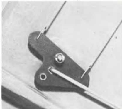
Pushrod fixed to bellcrank with 2 bend allows removal for adjustment, inner hole reduces sensitivity for learning. Double locknut essential on bellcrank pivot bolt.
