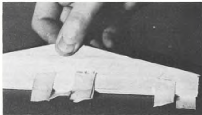
Cotton tape strips are used to hinge the elevator. Start by gluing them to the tail plane alternating above and below, before bending strips across the hinge line and adding the elevator. Avoid dope or paint on hinges from stiffening controls.
