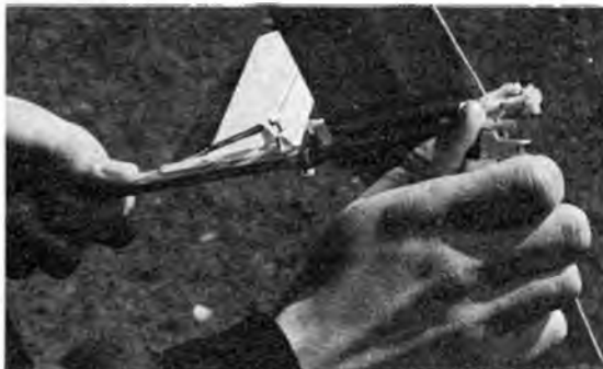
Above: Small piece of D.T. fuse, sufficient for 2 minute flight. Do not light directly as shown because of fire risk, instead light from fuse already smouldering.
