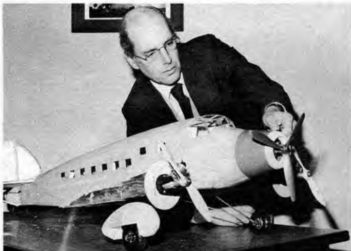
Control Line Scale Savoia-Marchetti SM 73 by Geoff Spriggs. Left: Model is powered by two PAW 19s and one Frog 3.49 BB diesel and is built with detachable wings to ease transport problems. Below: The design is scaled up from Aeromodeller FF Scale design FSP1077 by T. Potesta (price £2.75 inc. p&p), and with plenty of wing area and light loading should prove an ideal sedate flying scale subject.
