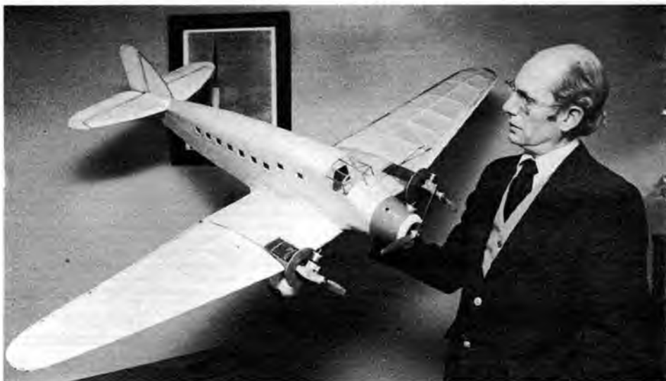
Control Line Scale Savoia-Marchetti SM 73 by Geoff Spriggs. Left: Model is powered by two PAW 19s and one Frog 3.49 BB diesel and is built with detachable wings to ease transport problems. Below: The design is scaled up from Aeromodeller FF Scale design FSP1077 by T. Potesta (price £2.75 inc. p&p), and with plenty of wing area and light loading should prove an ideal sedate flying scale subject.
