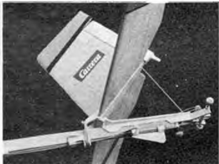
Pre formed plastic mouldings also used on Carrera Dax glider, enabling AR and DT to be assembled simply like any plastic construction kit. Left, line to clockwork DT timer at nose holds down tail; until line is released allowing tail to pop-up to 45°, right.
