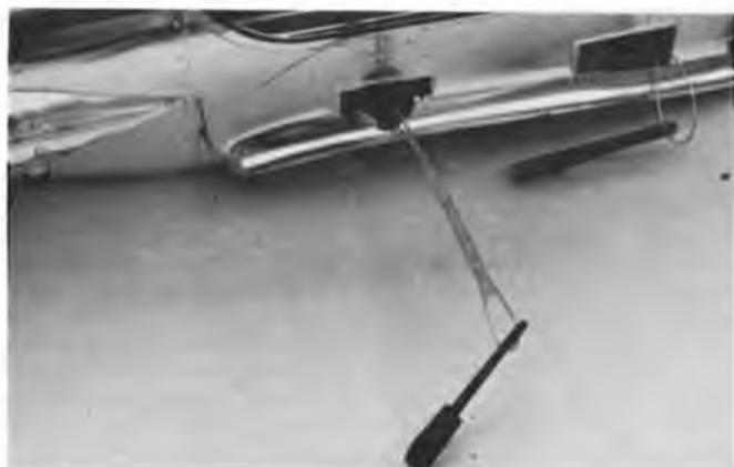
Top left: some of the Testors propellers, note the lugs for locating the spinner and the blunt blade tips for safety. Nose of the Cosmic Wind top right with the front part of the cowl removed. The Zip starter stick locates the cog behind the propeller and is held engaged while starting by the front cowl moulding. Right the leadout wires on the Silver Wind. Below left the engine installation. The very simple, but effective battery clip for Duracell batteries is shown below right, and in use, centre.
