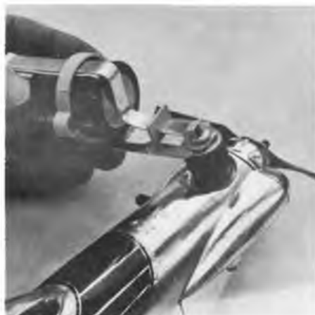
Top left: some of the Testors propellers, note the lugs for locating the spinner and the blunt blade tips for safety. Nose of the Cosmic Wind top right with the front part of the cowl removed. The Zip starter stick locates the cog behind the propeller and is held engaged while starting by the front cowl moulding. Right the leadout wires on the Silver Wind. Below left the engine installation. The very simple, but effective battery clip for Duracell batteries is shown below right, and in use, centre.
