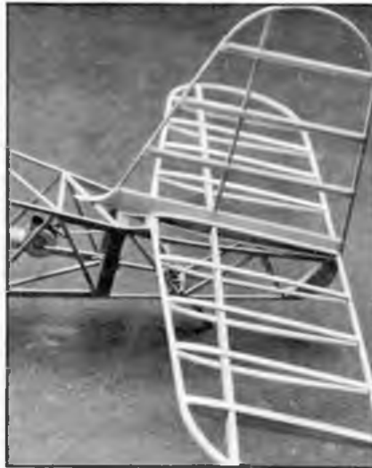
Left all spruce structure, papier-mache wheels and freewheeling propeller all combine to give Alan Crompton's Jackdaw a really convincing look. Above Alan's Jackdaw II built completely as per (see text) appropriately registered G-AEIN. Below close up of the Jackdaw stern showing the motor anchorage. Below right unknown modeller lets her go! Can any reader please tell us, who, what, where, when?
