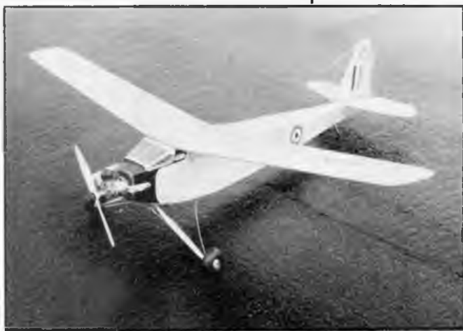
Left: this model was originally built during 1935-36 by Fred Rising, who powered it with a home made Westbury Kestrel 5cc petrol engine. The 66in span renovated model is now owned by A Askw and flown under radio control it relies on glow plug power. seen here at last year's Nationals.
