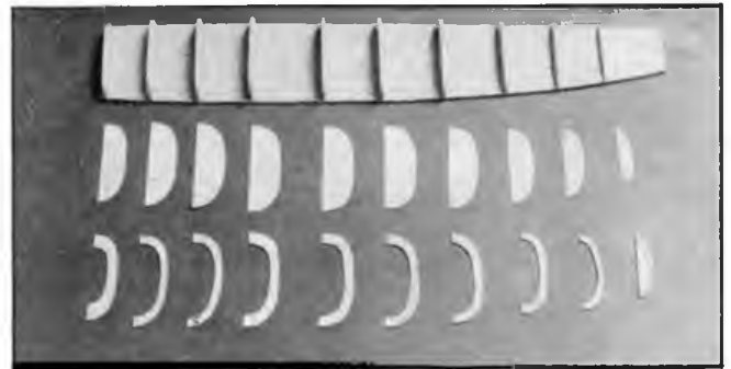
Left Peanut scale ultralight Brown 'Miss Los Angeles' racer is covered in condenser paper and weighs 9 grams with rubber motor. Above this jig was used for working out the shape of the fuselage formers on a Peanut scale Brown 'Miss Los Angeles' racer by the author (details in text)
