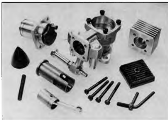
Parts of ball-bearing model Pfeffer 0.6. Note long stroke piston/liner assembly. Cylinder has twin opposed exhaust ports, long transfer channel at front and induction port at rear
