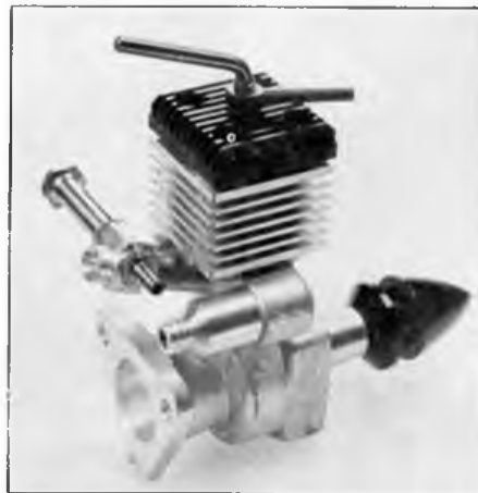
Left: parts of the newest ST35. Modern features include Perry supplementary ports and dual concentric bowl combustion chamber. Right: unmistakable features of Pfeiffer 0.6cc diesel are its square finned cylinder, built-in twin silencers and triangular mounting flange.
