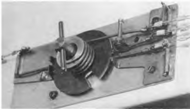
The Ray Monks built timer on Stafford Screen's F1C aircraft in the launch configuration. Note the Laystrate lines permanently attached to the timer arms, they pull tight via an over-centre action. The D/T arm (top right) is held down by the 8BA screw latch on the bunt arm, to prevent premature D/T action. Note also the locating slots to prevent circumferential movement of the arms caused by friction from the timer disc.
