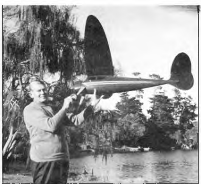
Bill Mackley of Auckland with his 6ft wingspan, Baby Cyclone powered T. Tailed Venus built and flown before the war, recently renovated and made airworthy
