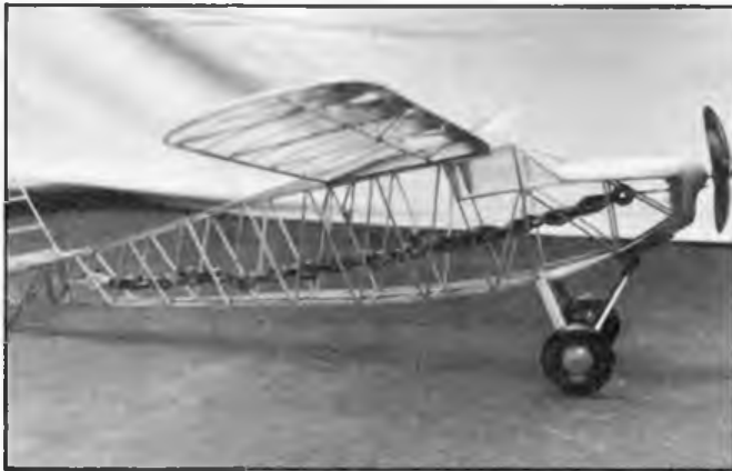
Left all spruce structure, papier-mache wheels and freewheeling propeller all combine to give Alan Crompton's Jackdaw a really convincing look. Above Alan's Jackdaw II built completely as per (see text) appropriately registered G-AEIN. Below close up of the Jackdaw stern showing the motor anchorage. Below right unknown modeller lets her go! Can any reader please tell us, who, what, where, when?
