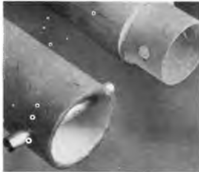
Rear boom to motor joint of Jedi Knight. Glass fibre tube fitted to both units for tight location and locked by motor peg.
