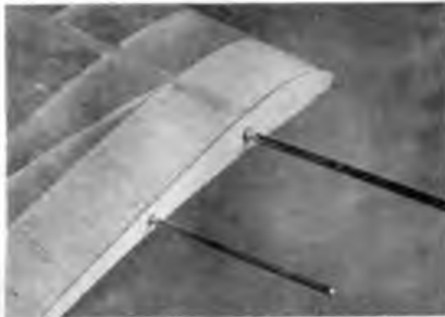
Wakefield wing half with wire joiners in position.
