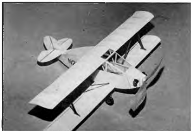
Dave Day's Peanut Sorrell Guppy ultralight built from Model Builder plan. Weighs 10 grams with rubber. Covering is Jap tissue sprayed with enamel over cellulose
