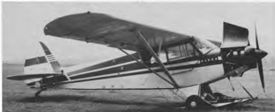
A BIPE? Yes - N43512 has a lower wing added and a heavy duty tailwheel unit. Origin of this oddity among PA-18-150's would be interesting. (Photo: A. Heape).
