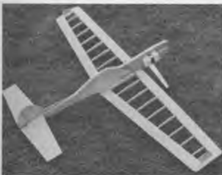
Above: power plant and fuel tank assembly, fine for training flight but 'Yeyito' could probably benefit from a small stunt tank. Left: finished model ready for covering. Right: just a small amount of trim tape will transform the looks of this smart model.
