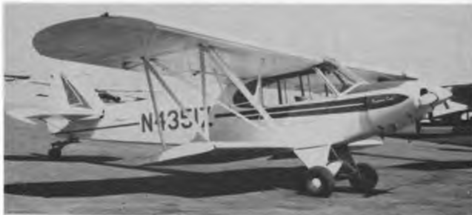
A BIPE? Yes - N43512 has a lower wing added and a heavy duty tailwheel unit. Origin of this oddity among PA-18-150's would be interesting. (Photo: A. Heape).
