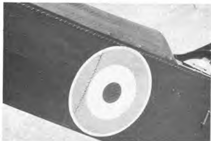
Above: John Coker's Sopwith 'Triplane' is worth another look before the covering goes on. Below: silk is doped onto the wing lower surface. Silk is tricky to keep in one place - note the initial spanwise stripe of dope. Right: the side of the author's 'FKB' shows the realistic fabric lacing effect obtained using a sewing machine as explained in the text.
