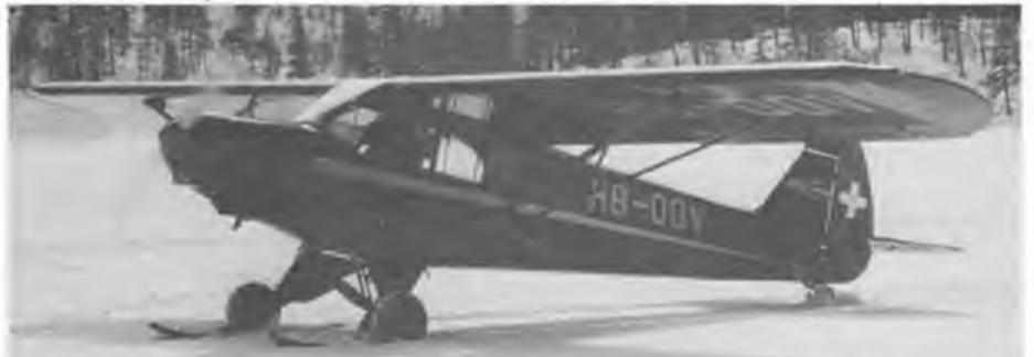
Two Swiss examples 'RAL (see text) has a Franklin engine and locally made wheel spats. 'OOV (below) in typical surroundings is on skis for the mountain rescue service which the 'Cubs' maintained for years until arrival of helicopters.
