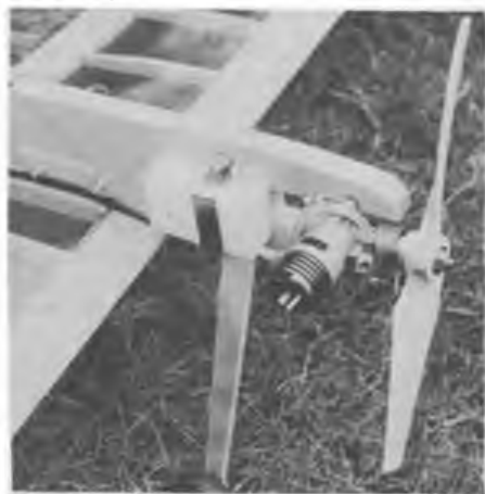
Above: power plant and fuel tank assembly, fine for training flight but 'Yeyito' could probably benefit from a small stunt tank. Left: finished model ready for covering. Right: just a small amount of trim tape will transform the looks of this smart model.
