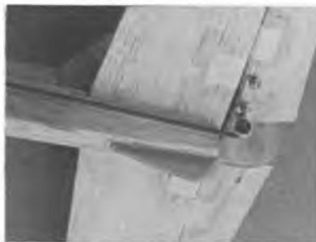
Left: inboard wing under construction, ribs are sanded to shape when glue is completely dry (24 hours). Right: close-up of simple undercarriage fixing, easy to remove if desired. Below left and right: fore and aft control linkages showing very straightforward method of attachment.
