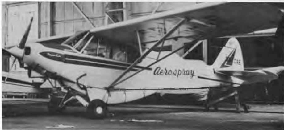
PA-18A 5B-CAE Cyprus registered agricultural variant with belly tank. Below: French ski equipped version retains the wheels and steerable tailwheel.
