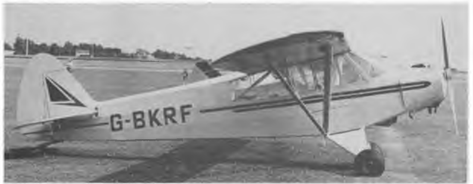
One of several newcomers to the British register, 'BKRF is a 'straight' L-18, ex Italy, and overhauled in the UK. Battery access panel behind glazing on St'bd side is a British modification.
