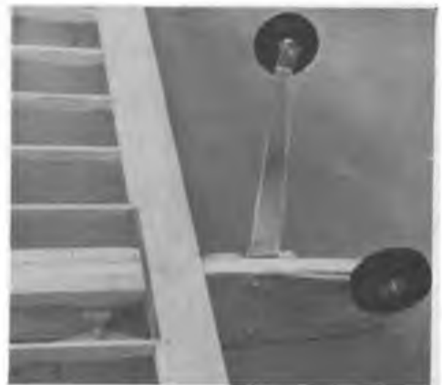
Left: inboard wing under construction, ribs are sanded to shape when glue is completely dry (24 hours). Right: close-up of simple undercarriage fixing, easy to remove if desired. Below left and right: fore and aft control linkages showing very straightforward method of attachment.
