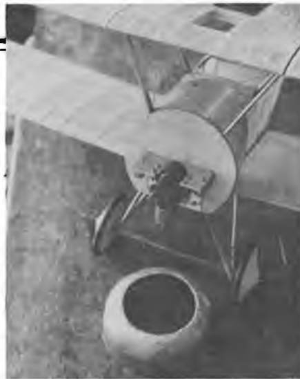
Above: by a stroke of luck, an aluminium teapot yields quite a good cowling and fits perfectly. Note the engine installation, the 'Mills' carburettor passes through a hole in the bulkhead.
