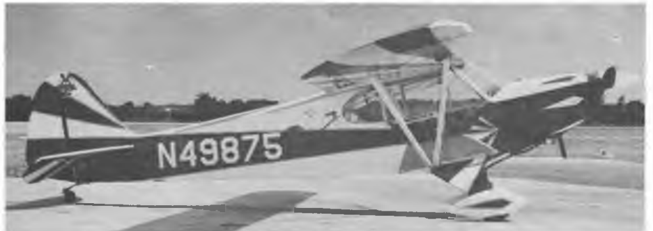
Long nose, sunray wing decor, and roadrunner markings ahead of N49875 reg'n give the clue that this is one of the re-worked aerobatic versions in the USA. (Photo: Erwin J. Bulban, Dallas).
