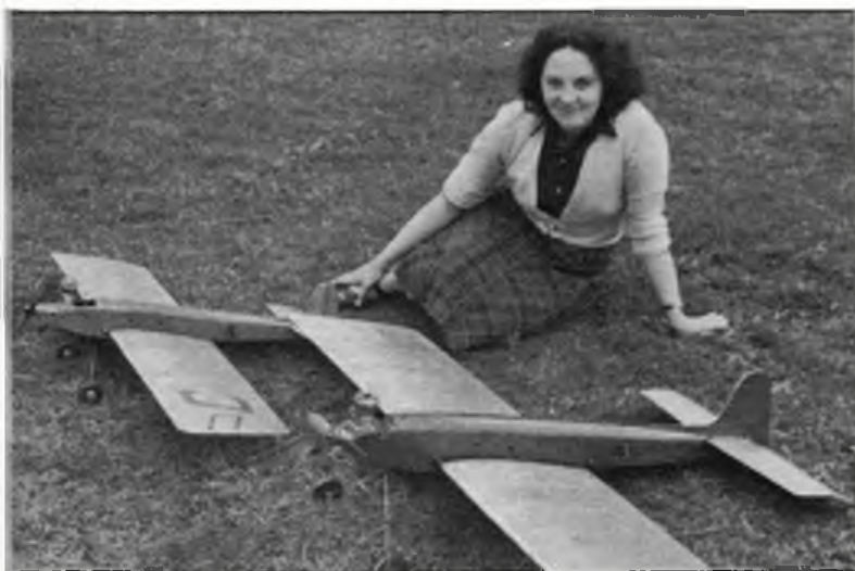
Bridget McCann with future husband Peter Russell's stunt design 'Barn Door' seen here in two versions 58 and 78 inch spans. The smaller started life with a Fox and ended up with a McCoy 60, larger version sports a Hornet and was fully aerobatic (1950's style) flying at 65 mph on 100ft lines.
