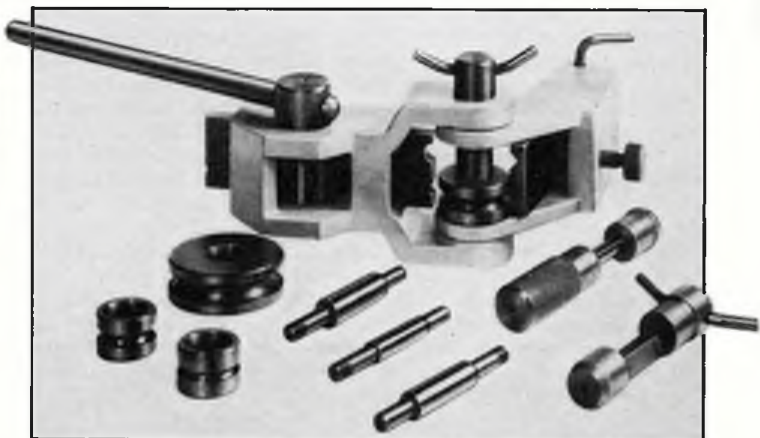
Below, the 'Universal Metal Bender' from C.Z. Scientific Instruments together with a selection of mandrels and grooving rollers. Left, some of the shapes that the 'Universal' can help you bend.
