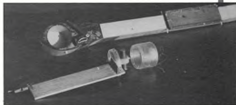
Above, steering unit out of its plastic 'pill box' showing the chunky bar magnet that does all the work. Left, steering unit installed in model, note unit may be removed for installation in second (third?) model.
