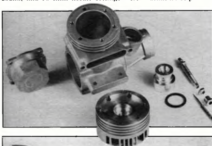
Left and below, once disassembled the Como 51 discloses well machined and finished components suggesting a long and reliable life when installed in a stunt model.
