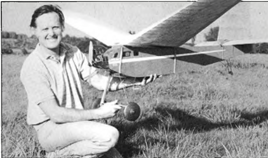
Nice study of Tony Penhall's replica 'Blue Dragon' taken by John Kemp. Undercarriage leg fairings are slats of wood 1/4 inches wide wrapped with silk; note that Tony has lost the fairing on the port leg during trimming flights. The engine is a 1938 Brown Junior Model D with the simple needle valve at the extreme end of the intake tube.
