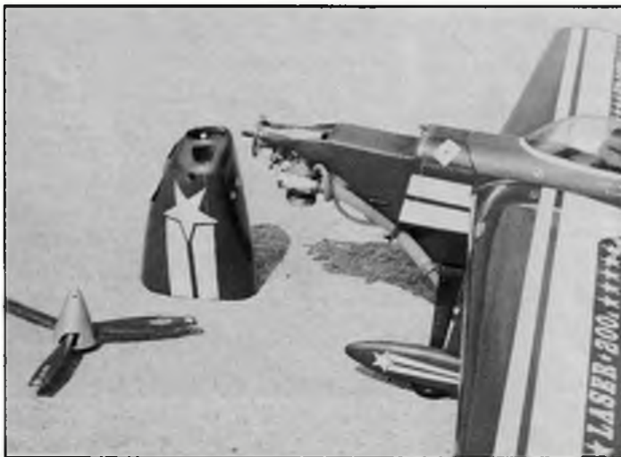
Above, upside down with nothing on the clock! Yves Fernandez Super Tigre ST60 powered 'Miles' with close-up of sprung undercarriage arrangement and flap horn connector at top right. At left and below, the sparkling Laser 200 of Polish stunt maestro Piotr Zawanda. Cowling and wheel pants are home-moulded from glass fibre (see text) and model is Super Tigre 46 powered with cut down Rev-Up three blade prop.
