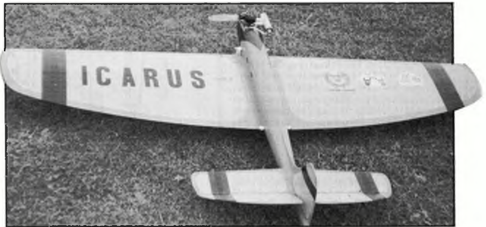
Above, John Parry's version of streamlined stunter 'Icarus' published in Aeromodeller in April 1951. Two plans were available, one for 42 in span (5cc) and the other 67 in span (10cc). This is a larger version and is powered by a Fox 59.
