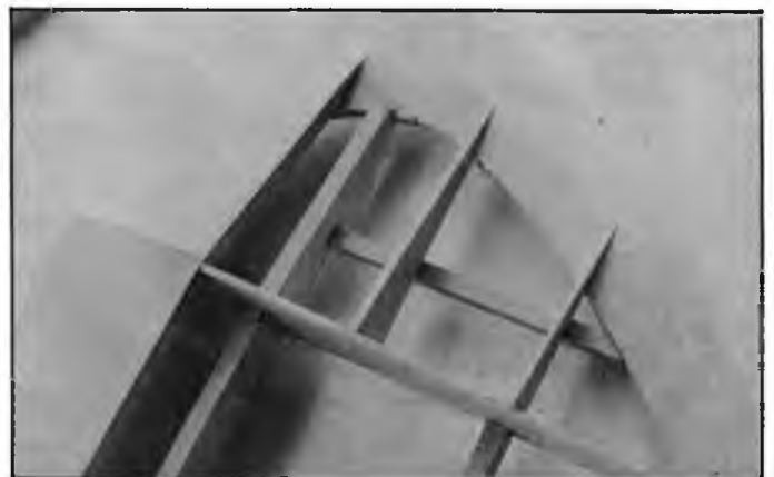
Close-up of wing tip showing triangular webs to support covering; leading edge sheathing has also been extended onto the tip.
