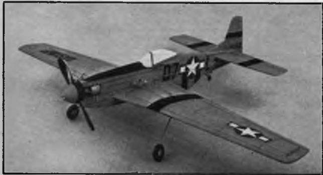
MUSTANG — SPAN 37¾" for .15 CU.IN. ENGINES
