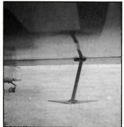
Su-26 detail to help the modeller. All photos are of '07', captured by Pat Lloyd at South Cerney. Left: Vest cowling reveals the powerful M-16P radial, geared down to drive that broad-blade prop. Below: Triangular aileron attachment reduces stick load. Significant roll rate was reported by observers of this aircraft. Middle left: Disc brakes are prominent; single-leaf undercarriage is from titanium. Middle right: Wing fillet is the only obstruction to all-round vision. Attached to the port wingtips is a positioning guide. Bottom left: Rear-hinged canopy opens to reveal Soviet Team member Nikituk checking his Aresll aerobatic programme. Bottom right: Steerable tailwheel assembly is another robust fitting.
