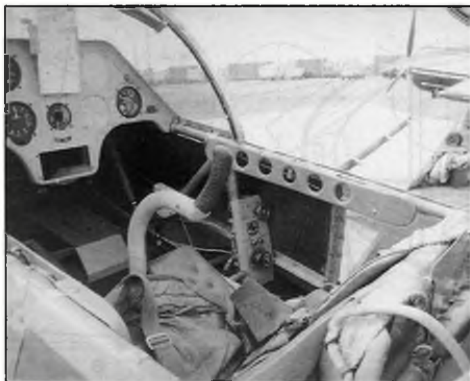
Cockpit shots indicate differences between '01' (main picture) and '07' - joystick and instrument panel, for example! Photo at top left reveals common mounting of throttle and prop pitch control - throttle inboard. Note also shield for rudder cable fitted to diagonal tubular member. Photos: Otokar (01) and Pat Lloyd.
