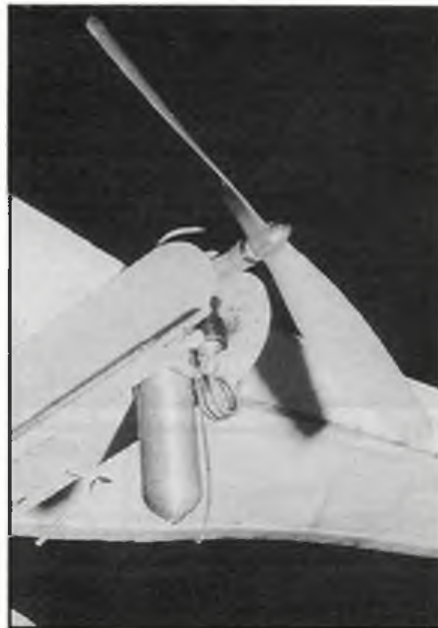
Below: Two views of the inverted Modella. Throttle control is effected by pushrod-actuated rotation of cylinder barrel (the full story next month!). Wire skid is prominent.
