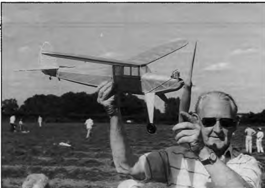
The rarely seen Scientific Firefly, a gas-type free-flight rubber model. The dummy engine looks convincing; motor hum ratchet on the prop shaft provides the sound effects. The size of the prop is the give-away! Model is the work of Tom Rostron of Poole.
