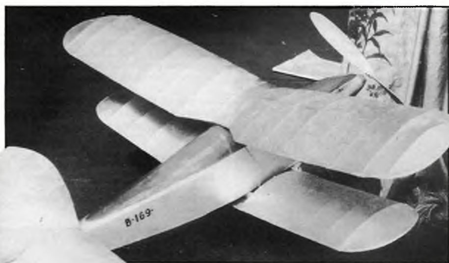
C E Bowden's rubber powered Fox, of 39 inches span and weighing seven ounces was one of three models that he showed on the SMAE stand at the 1931 Model Engineer Exhibition.
