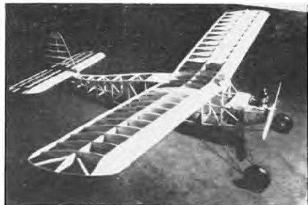
The "Cloud Airmaster," 7 ft. span, powered with a 9 cc. Ohlsson engine, built by Mr. A. B. Stevens, a member of the Woking and District M.A.C.
