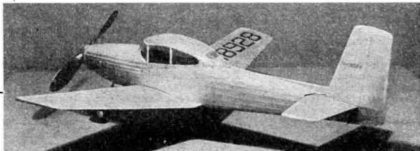
The original Navion was incorrectly fitted with a spinner, as shown here, but later versions had the scale type prop shown on the plan opposite.
