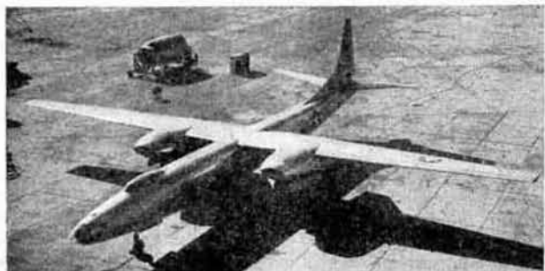
FLYING PENCIL. Below is the Convair XB-46 medium bomber fitted with four jets and having a wing span of 113 ft. (Convair Photo.)
