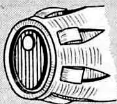
FIG. 4. COWLING SHAPE FOR ROLLS-ROYCE KESTREL ENGINE.
