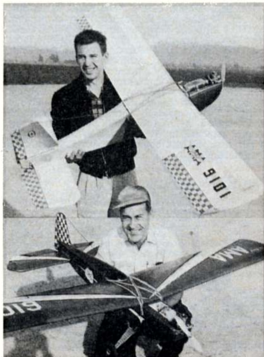
Left: Fergus O'Brien's scale Skylark is 10-ft. span. Below: Bill Verney's Superhet to Dave McQue's design weighs 5½ oz. Oper- ates on 7\frac{1}{2} to 9 v.
