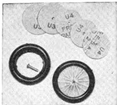
Frog SE5a wheels take full marks for good ideas. Have plastic tires, brass bush and fabric over "spokes"
