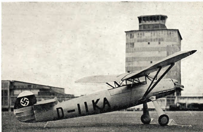
March cover, showing the A.P.S. Fokker Friendship by Maurice Bodey on the apron in front of Liverpool Airport Control Tower inspired M. A. Hundley of Hazel Grove, Cheshire, to produce this picture. It shows his 34½ in. Focke-Wulf Stösser to 1/12th scale posed at Manchester Airport. The model is powered by a Mills .75 c.c. diesel with only the compression screw exposed. Its fuselage is planked with ¼th balsa sheet and the wing is in one piece, held to the centre section cabane by rubber bands.
