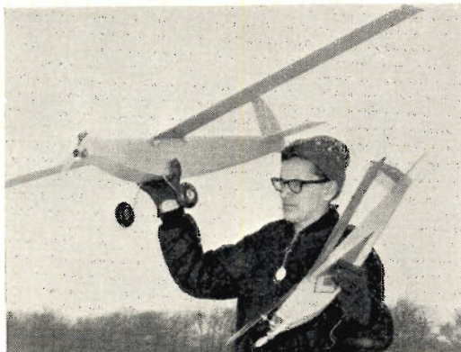
Jimmy Stouffer holds two versions of SIMPLEX, 6 ft. span and the 36 in. span. The proportions are the same. Both are rudder only with .049 O.K. Cub and .19 rear rotary McCoy engines. Weight of the larger model is about 3½ pounds. An Ecktronics Kraft single channel receiver is installed, 3.6 volt Nickel Cadmium cells provide electrical power for the Babcock escapement operation. Wings are carved from ¼ x 6 x 36 in. soft balsa and joined at the dihedral point with multiple layers of glass fibre and resin.
