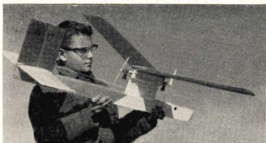
Cylinders separated! Push-pull twin .049 glow plug engines powered Mark III as a variation on the "Simple Simon" theme—with radio control.
