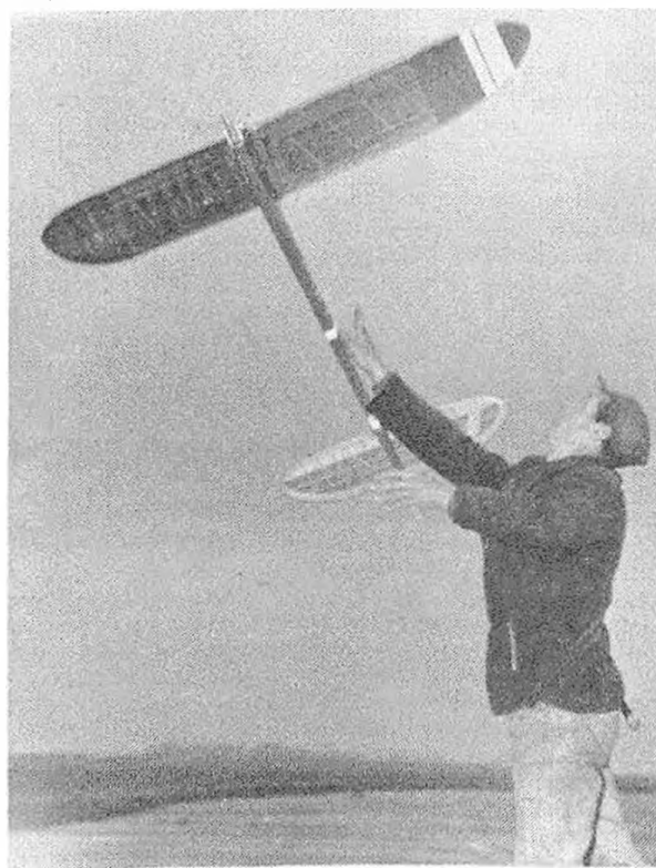
Joe's launching tip is to point the model 15-20 deg. to the right of the wind direction in order to achieve maximum rate of climb. This typical hand launch following an underarm launching action shows how the designer starts 'Faital' on its upward way.
