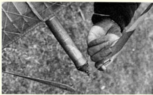
Detail photo of Arthur Schaffler's nose assembly shows use of outrigger prop. A 3-D saw-toothed turbulator is used on the wing, and note also thread on top of wing tissue.
