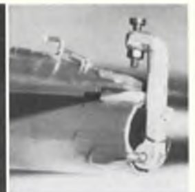
Above: At the 'other end', the VIT arm is in position, and the tail is held down on to the lower stop (for initial 3 seconds). The screw is for glide adjustment. At left is result of D/T being actuated - note how VIT arm springs backwards.
