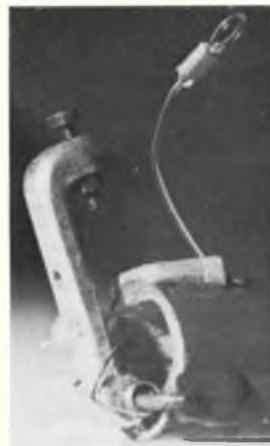
Above: At the 'other end', the VIT arm is in position, and the tail is held down on to the lower stop (for initial 3 seconds). The screw is for glide adjustment. At left is result of D/T being actuated - note how VIT arm springs backwards.
