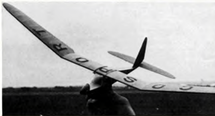
The Tern 'Traveler' has a remarkable performance for such a small glider, and proved very stable on the towline. High aspect ratio wing with tapered tips help add to the attractive semi-scale appearance.
