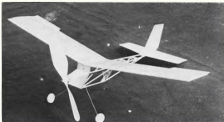
Built by our reviewer in under two hours, the 'Aerobug' proved a really robust rubber-powered sportster with a creditable flight performance - once more rubber had been added. Easy to trim, and definitely non-critical.
