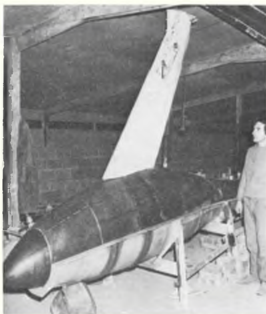
Peter Wright of Melton Mowbray is completing his second MP aircraft which, like his first, employs carbon fibre-reinforced epoxy extensively. In fact, the 'Micron' is almost all plastic and has been produced in moulds so that others can be made later. Aspect ratio is 'over 40:1', and the vee-tail has butterfly rudder-ventrator controls. The 'Micron' will have a 9ft. diameter propeller and what promises to be high efficiency performance from the narrowest wing yet seen on a man-powered aircraft. The whole design and construction has been a solo effort and included making the scale test model which Peter is seen holding at the Royal Aeronautical Society Symposium.
