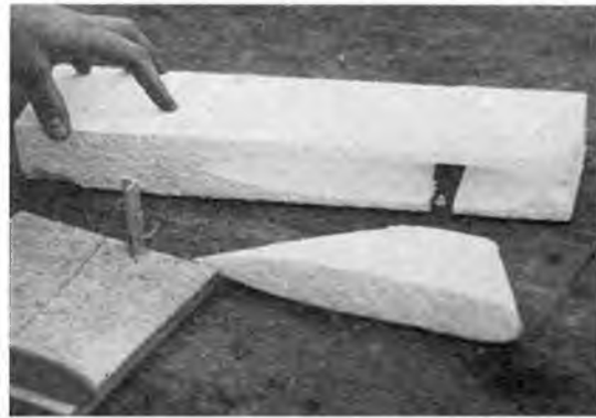
After cutting wire has reached point '6' (Figure 6) the same scrap piece is lifted away and the formed tip will fold away free. Save all scrap material for making these tips.
