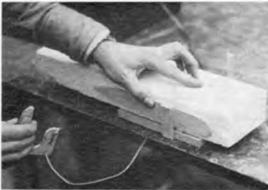
Large foam tips are light, aerodynamically more efficient than most currently employed - and easily cut out. Here the hot cutter wire (drawn in Figure 5) is being taken around the template.
