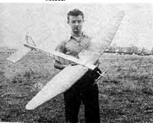
Rudolf Lindner's Spinne (Spider) which gave W. Germany the 1954 A/2 victory. Abolition of the 'fuselage formula' meant only a slim rod to carry wing and tail was needed.
