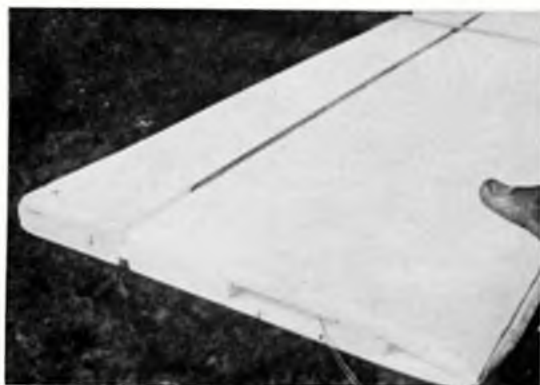
End view of incomplete wing reveals simple construction and method of obtaining the hollow 'core'. Note too the 'groove' for spars and leadout wires exiting from the core. Flat wing section has long been favoured by combat fliers.
