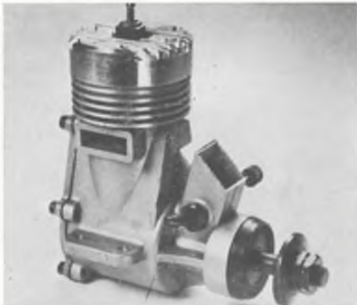
The latest of a long line of Fox Combat-Specials. The first Combat-Special appeared 20 years ago. Latest Mk. III model features Schnuerle porting and twin ball bearings. Capacity: 0.5594 cu. in. or 5.889 cc.
