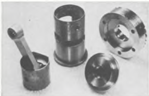
Fox has lapped cast-iron piston running in steel liner. New type head provides for interchangeable inserts for different compression ratios.
