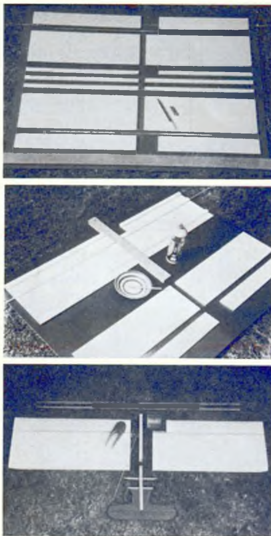
Top picture shows the basic materials necessary for producing a model from polystyrene ceiling tiles, namely a straight edge, 30°-40° set square, felt pen, 'Stanley' knife and the tiles themselves cut for inboard and outboard panels – the leading edge pieces being shorter to accept engine pod and fuel tank. Centre picture shows building two wing panels together. The lower parts of the centre strips are glued in place – note space for pod/tank. Also note two separate spars used, NOT running through the 2 x 1in block. Bottom picture shows HP3 ready for final assembly of the wing panels.
