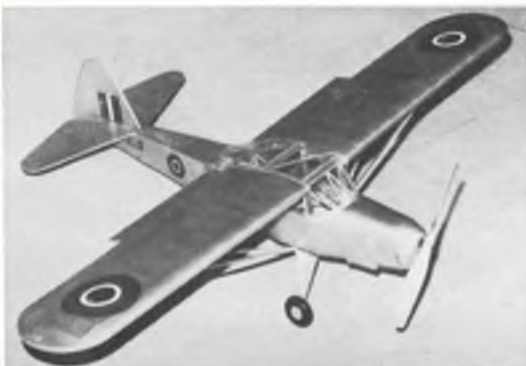
A 1/18th scale Auster AOP - by Derek Knight, converted from his own-designed rubber model to Telco CO 2 power. Very nicely detailed and finished.
