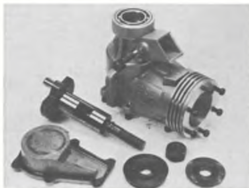
New Fox Combat-Special has tall back cover as used on current 15, 40 and 45 models. Note also massive unrestricted air intake.
