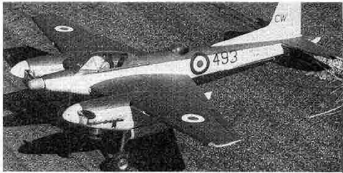
Albert Briggs DHC Hornet uses two throttled Oliver Tigers electrically operated by 3 line control, third at last years Nationals.
