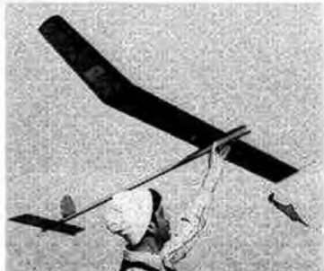
Sam Banerjee displays his G-90 A/2, asymmetric wing using all moving fin and offset towhook.
