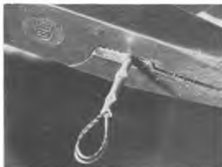
Above: Soft metal tubes crimped to hold looped ends, must be sealed with solder or epoxy to prevent lines slipping. Double loops add strength at point of wear, another point of safety.
