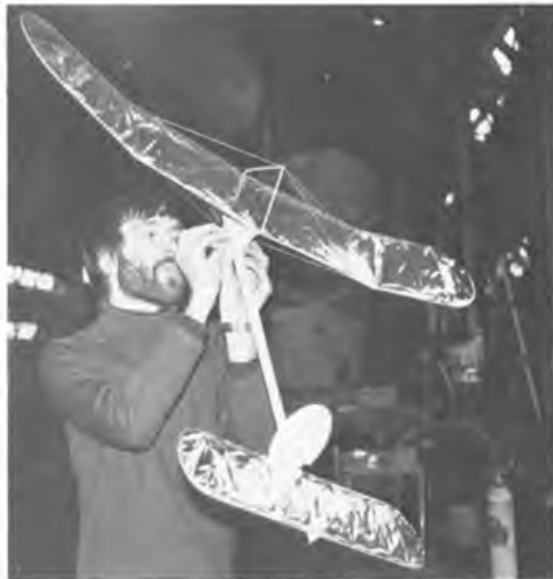
Above left: Derek Richard's duration model uses strong wing requiring no bracing. Above: Dave Hipperson favours super light approach, 42in x 6in mylar covered wing depends on cotton bracing lines to take flight loads. Below: 'From the sublime to the ridiculous,' Ron Green couldn't believe his eyes after Tim Gray produced this creation. Built the night before, it hit the roof 180ft overhead after about one minute and regularly turned in two minute plus times.
