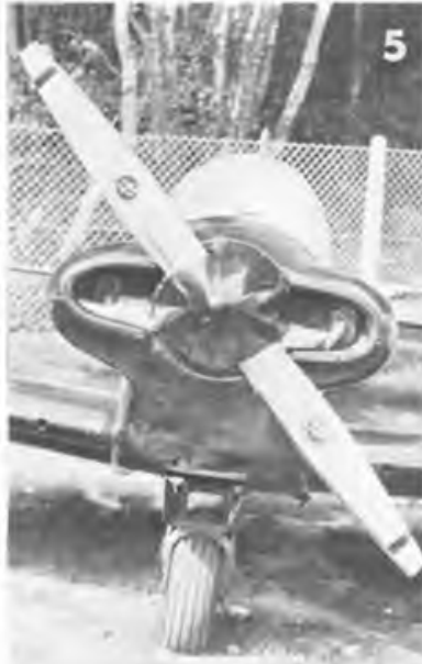
5. Hoffman prop has trademarks on each blade. Cowlings are slightly different Port and Starboard due to staggered cylinders. 6. Wheel close up, plus two external skids (in case of wheel failure!) Wire guides either side of wheel yoke open the spring loaded doors. White area is engine air outlet. 7. Rear of cockpit, red cushion on black vinyl, seat luggage area has extinguisher clip and radio. Constructor's number plate on bulkhead at top
