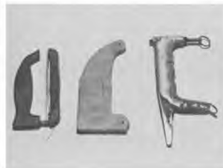
Left: Terylene lines stored on a lightweight Keil Kraft handle which has variable line spacing. Middle: Simple home made handle from 1/4 in ply. Right: D.C. handle with adjuster on top line.
