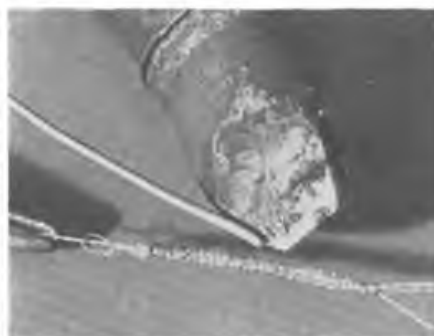
Above: Loops formed by binding with thin fuse wire before soldering. Neutralise flux after soldering by washing with baking soda solution to prevent corrosion from weakening lines.
