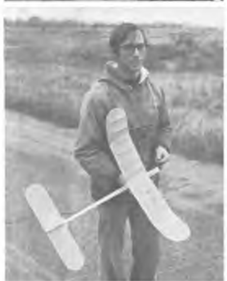
Left: Matin Simkins testing out his CO 2 outdoor model, built up wing uses thin undercambered airfoil as used on French Coupe designs, tail is built up flat plate. Fuselage, as seen above, uses longeron and spacer construction using 1/4in sq balsa, triangular cross section encloses fuel tank underwing. Right: Ray Pavely flew his outdoor CO 2 model at last year's Silent Gala, parasol mounted wing and extra large tail area.
