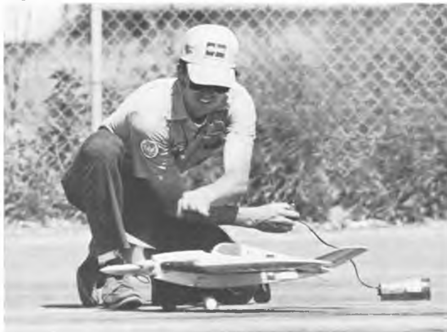
GOODYEAR – BAD YEAR! – BIG YEAR? America's answer to the excessive speeds of current rule models is their Big Goodyear class with 1/16th instead of 1/8th scale. Models worked out to 28–38 inch span, 260 sq in approx area and 28–35in fuselages. Above is Ron Duly's Sweet Pea which uses a built-up, rib and spar wing, and there he is in pristop action below. No hot gloves, pressure refills or fuel cut-outs are allowed to put back some simplicity in the racing.
