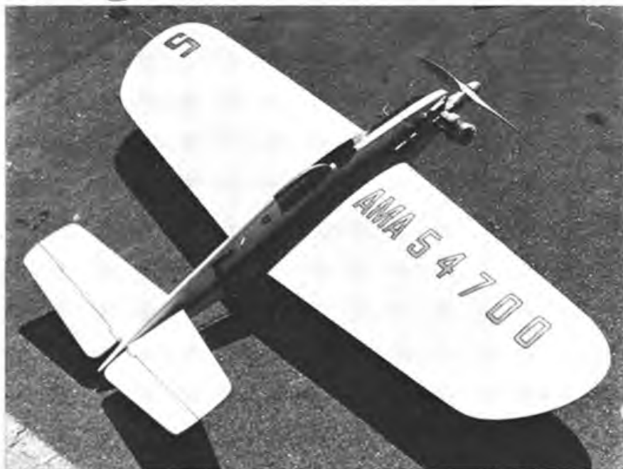
GOODYEAR – BAD YEAR! – BIG YEAR? America's answer to the excessive speeds of current rule models is their Big Goodyear class with 1/16th instead of 1/8th scale. Models worked out to 28–38 inch span, 260 sq in approx area and 28–35in fuselages. Above is Ron Duly's Sweet Pea which uses a built-up, rib and spar wing, and there he is in pristop action below. No hot gloves, pressure refills or fuel cut-outs are allowed to put back some simplicity in the racing.
