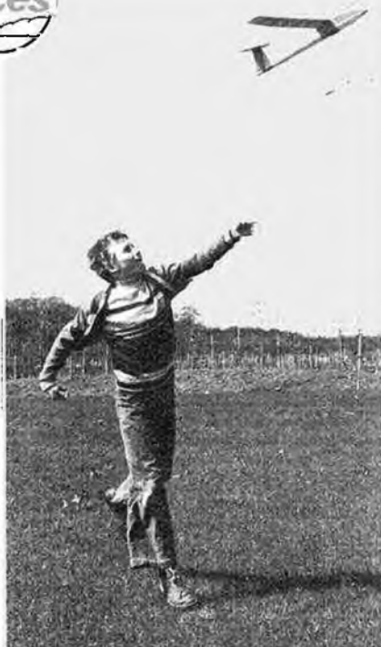
For towline launches, get a helper to release the glider. Hold the model with wings horizontal, nose up 30°, run with model and allow to lift out of grasp.
