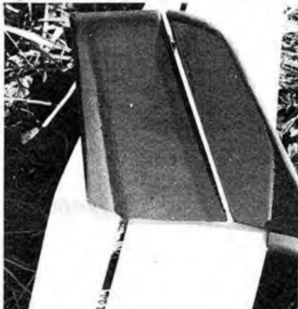
Above: something definitely to avoid, those yawning gaps between fixed and movable surfaces can reduce control response to a dangerously low level. Any gaps should be reduced to a minimum by close fitting surfaces or sealed with flexible iron-on covering.
