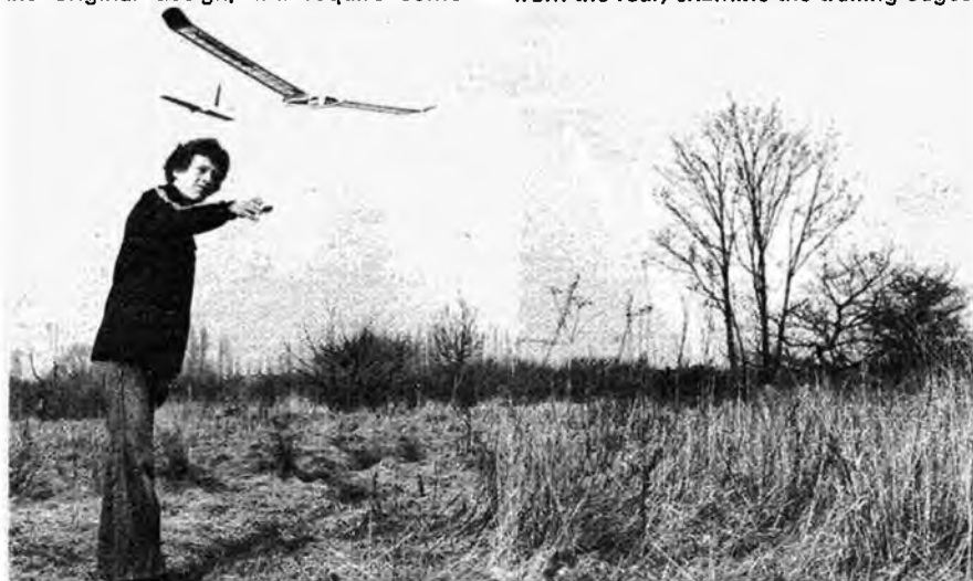
Above: test gliding the Graupner UHU, an ideal first model. Choose a calm day and face into wind, gently launch from shoulder height and follow through – like throwing a dart in slow motion. A long slow glide should result, but look for any signs of diving, stalling or excessive turning.
