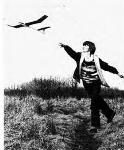
Above: The deliberate mistake – definitely NOT the way to test glide a model. A glider cannot possibly continue this upward path and will inevitably stall and dive into the ground – therefore choose long grass to fly over and launch more slowly, slightly nose down.
