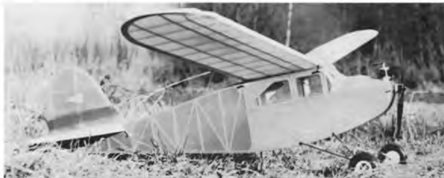
Below: JC 'Jenny' (span 72in), a design available from 'Power Models' of Southsea in the late forties, seen at Biggleswade resting between flights. This version powered by a Cameron 23 spark ignition engine was built by John Kemp, and is a regular performer at vintage meetings.
