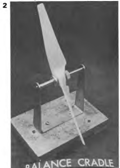
Right: propeller mounted in a balance cradle to establish static balance.
