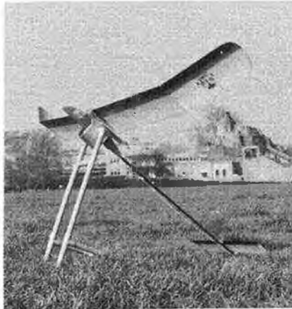
Right: ensure the launcher is held down firmly with substantial pegs.
