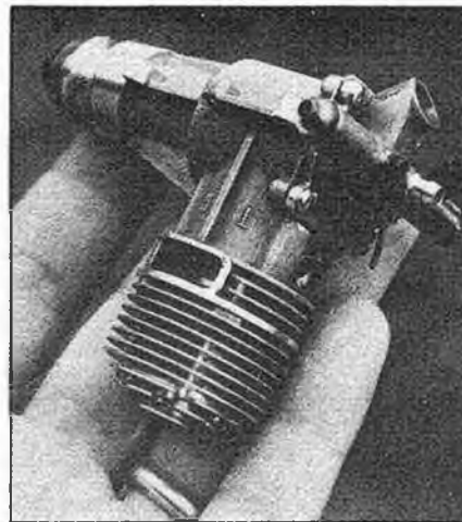
The CB2-5D (1980) diesel has six mounting lugs and bolt direct to the fuselage moulding.
