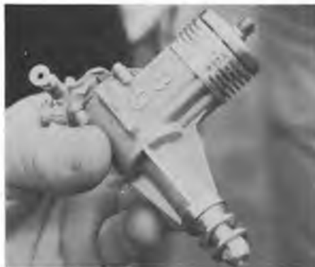
The latest version of the Danish BG engine, development of the late Paul Bugl's 15D. This is the version used to power the 'Klotzbug' - sketch plans of which appeared in December 1983. The case is stronger than the earlier versions with eight head bolts used to minimise distortion. Sadly the engine is no longer on sale to the public as the Danish enthusiasts could not find reliable production facilities.
