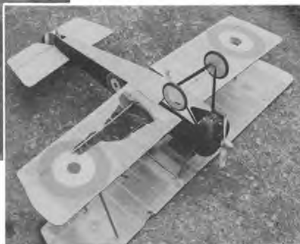
Above: the Puss Moth being test glided. Take care to always launch the model on an even keel. Right: the Sopwith 'Pup' after being brought down from the tree by rocks. Note that although the ribs have gone, the spars remain intact!
