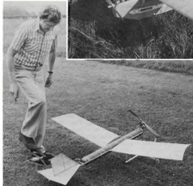
Above left: although HJN's 'Cloud Chaser' design was never published, D. M. Barton unearthed information enabling him to build this diesel-powered, rudder-only, radio-assist version seen at Old Warden. Left: Howard Boys with his tailless entry in the 1948 Bowden Contest at Fairlop, although he did not place in this competition, the 1.2cc Foursome diesel-powered flying wing was a consistent flyer and components survive today in use on Howard's experimental models.
