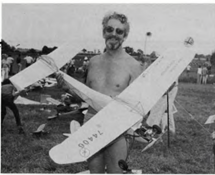
Above left: although HJN's 'Cloud Chaser' design was never published, D. M. Barton unearthed information enabling him to build this diesel-powered, rudder-only, radio-assist version seen at Old Warden. Left: Howard Boys with his tailless entry in the 1948 Bowden Contest at Fairlop, although he did not place in this competition, the 1.2cc Foursome diesel-powered flying wing was a consistent flyer and components survive today in use on Howard's experimental models.
