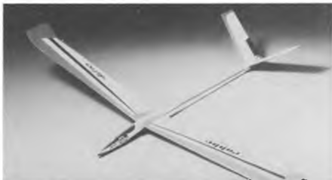
Two highly prefabricated kits from Robbe , above 'Fantra' the smaller of the pair at 28in. span and right the 'Astro' A1 class, at 57in. wingspan.
