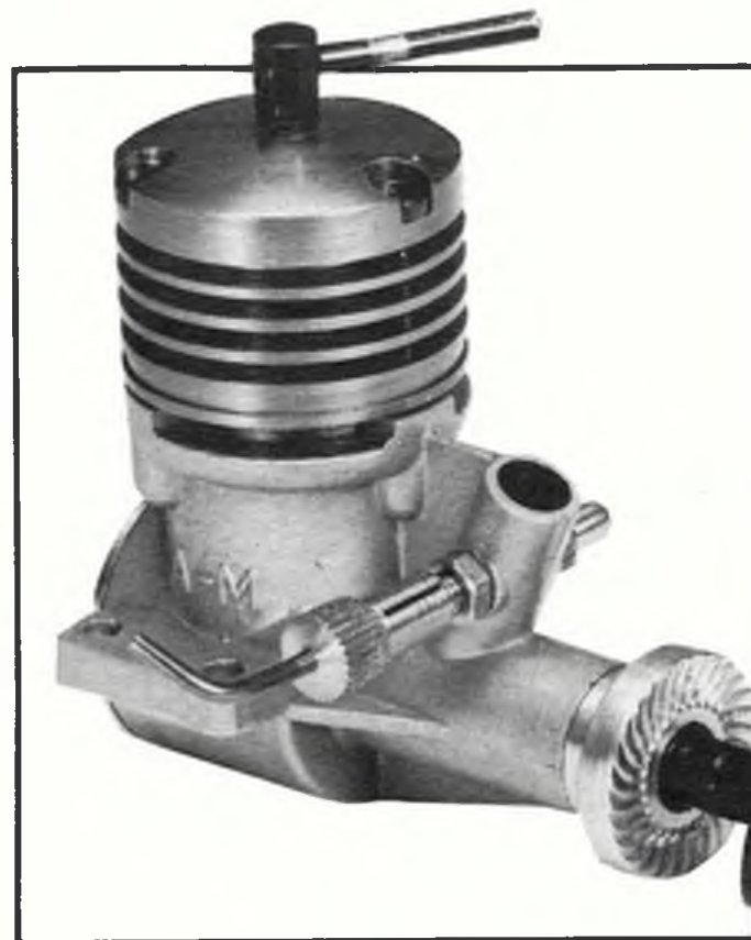
Left, on the review engine the compression screw proved to be quite hard to turn but by carefully tapping the tommy-bar it proved possible to improve matters as can be seen here. Remove the compression screw from the engine if you wish to try this, DO NOT tap (hammer) the tommy bar whilst still screwed into the cylinder head! It might be worth buying a spare (cheap enough ...) before attempting this mod!
