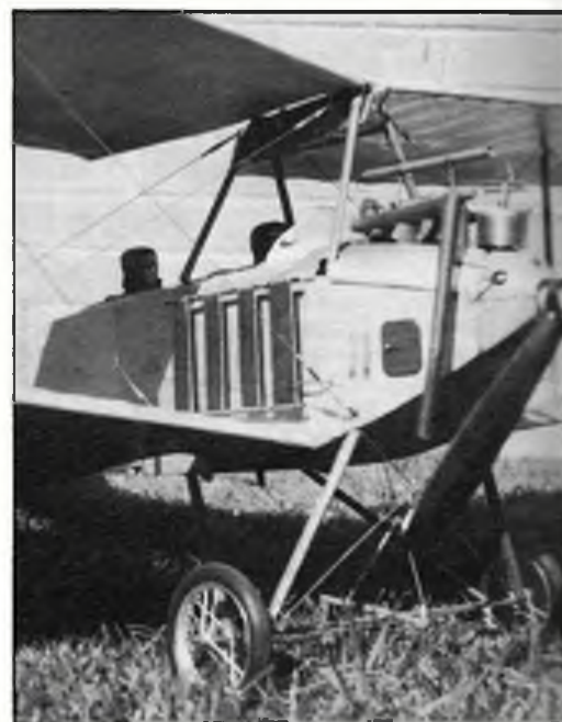
An Albatros B II by Gary Sunderland (Australia) to 1/8 scale. The fuselage is built from a laminion of 1/32 in. balsa and thin veneer.
