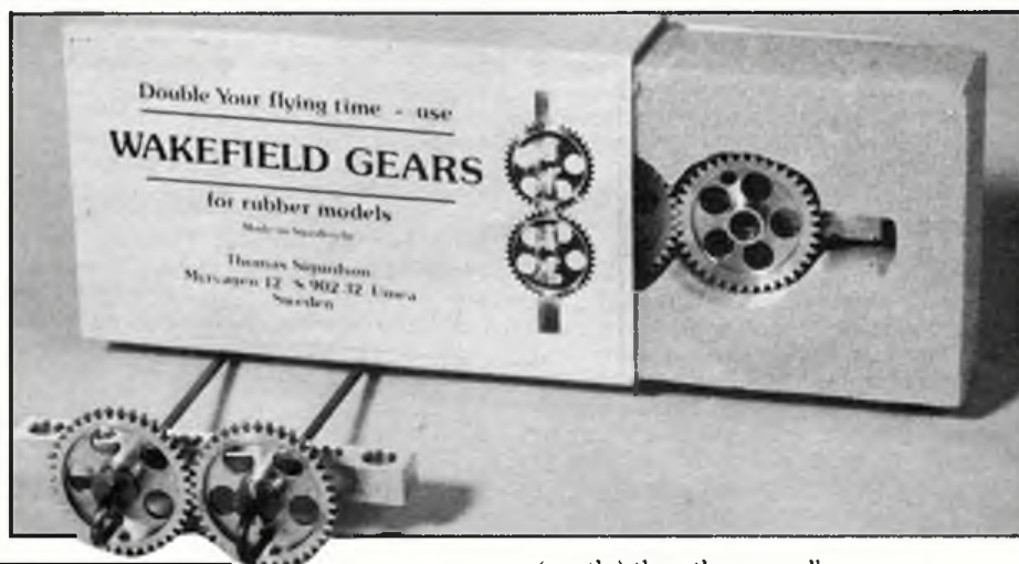
Above, quality return gear unit made in steel and aluminium by oldtimer-modeller Thomas Sigurdson from Sweden, just the job for that 'Ellila Wakefield'! (See text). Left, Another Stouffer shot: Bruce Norman hand launching his Ohlsson 23 powered "So Long" a Bill Englehardt design that was described in Air Trails , January 1941. This is one of the hottest machines in Class B Free Flight Cabin. Below, John Tidey, Secretary of SAM-Australia, sends this photo of his 6 feet span Modelcraft 'Spook', not a common model, due possibly to
