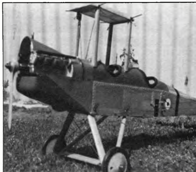
This free flight BE 2c by Gary Sunderland is one eighth scale, with a 2.5 cc Taipan diesel and working controls. Placed third at the Australian Nationals.
