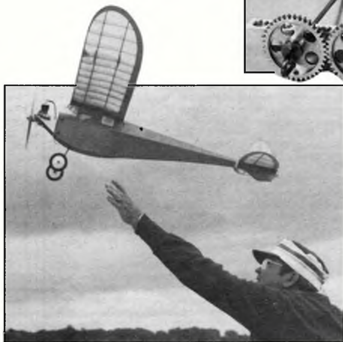
Above, quality return gear unit made in steel and aluminium by oldtimer-modeller Thomas Sigurdson from Sweden, just the job for that 'Ellila Wakefield'! (See text). Left, Another Stouffer shot: Bruce Norman hand launching his Ohlsson 23 powered "So Long" a Bill Englehardt design that was described in Air Trails , January 1941. This is one of the hottest machines in Class B Free Flight Cabin. Below, John Tidey, Secretary of SAM-Australia, sends this photo of his 6 feet span Modelcraft 'Spook', not a common model, due possibly to
