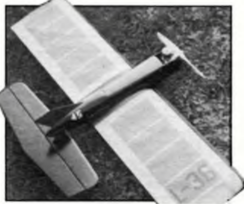
'Blue Pants', designed by Henri Stouffs for 2.5 to 3.5 cc engines was a 'thick wing' stunter flown in the 1954 World Control Line Champs in Holland. Span 39 inches.
