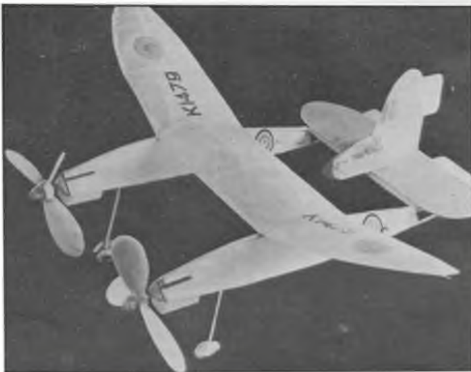
Below left, 'Demon' twin-motor semi-scale RTP rubber model designed June 1946, this photograph appeared in his own 'Model News' in January 1948 Aeromodeller with suitable comment! Below right, 'Mamba Mk I', 34 inch span, weight 5 oz. A most successful flier in both free flight and RTP, each motor was 6 strands 17 inches long of 3/16 in rubber, free-wheels were completely enclosed in the large diameter spinners.
