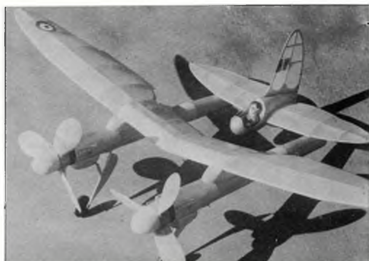
Below left, 'Demon' twin-motor semi-scale RTP rubber model designed June 1946, this photograph appeared in his own 'Model News' in January 1948 Aeromodeller with suitable comment! Below right, 'Mamba Mk I', 34 inch span, weight 5 oz. A most successful flier in both free flight and RTP, each motor was 6 strands 17 inches long of 3/16 in rubber, free-wheels were completely enclosed in the large diameter spinners.
