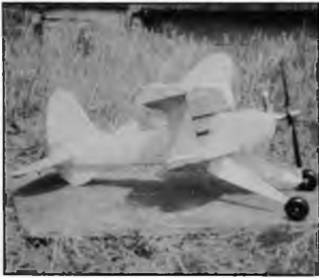
Above, 'Mentor Mk I' control line primary trainer for the Amco .87 diesel was designed and built July/August 1947 and weighed 6½ oz. Ray commented "...light on the lines, control poor since model climbed too well..."
