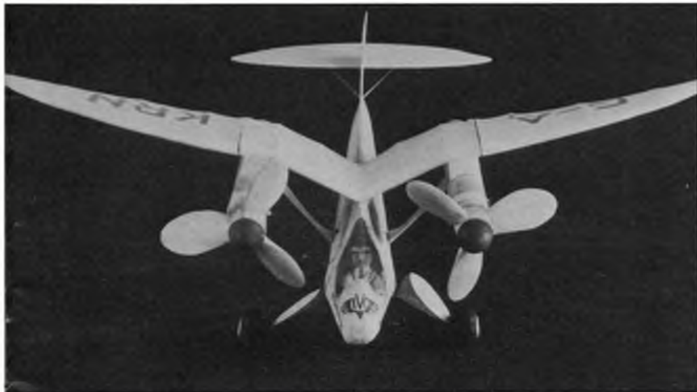
Above, 'Meanderer' twin-engined 3-seat light aircraft used monocoque engine nacelles and a papier-mache cabin unit, a steady and consistent RTP performer. Below, 'Skyrda' 31 in span free-flight model was described in American Aircraft Modeller magazine, powered by the Cox 'Pee Wee' 020 glow plug engine.
