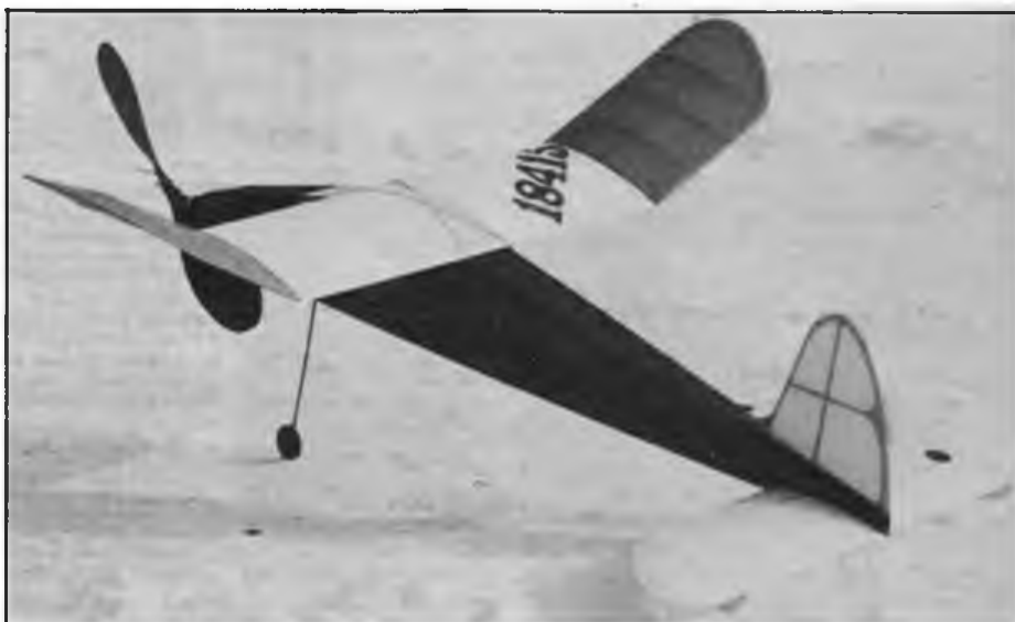
Above, during the winter, Dave had time to build this 'Senator' from an original plan supplied by Mike Kemp. Weighs 80 grams including 30 grams of FAI Supples rubber. With a 13in treewheel prop it climbs for over a minute and has already exceeded 3 minutes in sub zero conditions.
