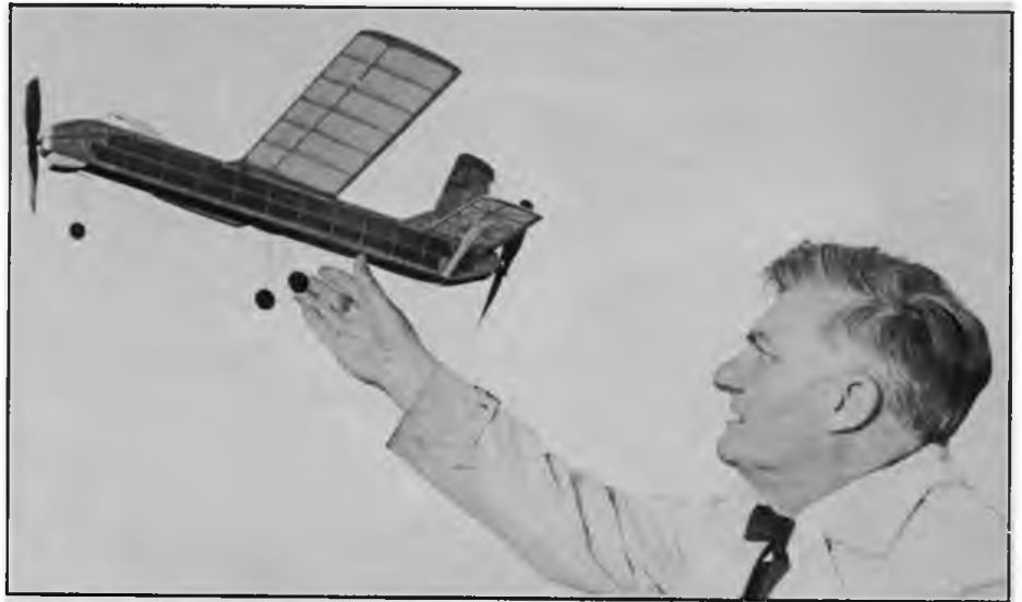
Above, Fliar Phil himself Ray launches his excellent performing 'Coaxair' 26 inch span rubber model fitted with coaxial propellers.
