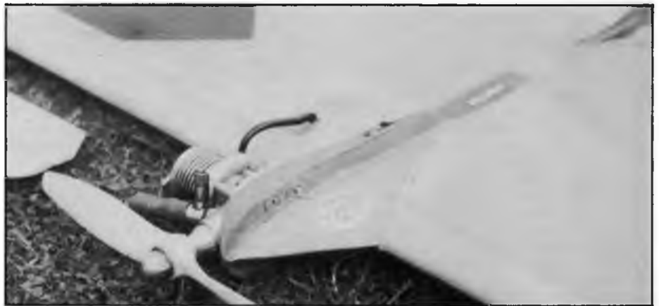
Above, not only does Frank Smart's engine pod add to the strength of the engine bearers but it looks good and reduces the drag!
