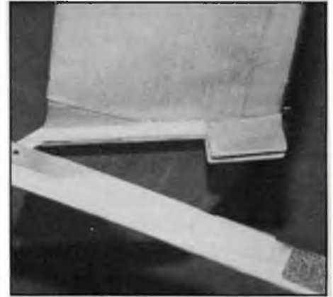
Above, wing in dethermalised position. There is no tension band or spring - so pivot must be very free...
