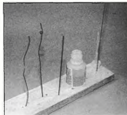
Cyano bottle safely housed in small balsa plank which doubles as 'pin cushion' for the applicator sticks.
