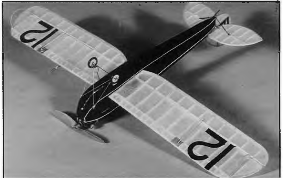
Details such as aileron linkage and wingtip skids add authenticity; weight increase is negligible.
