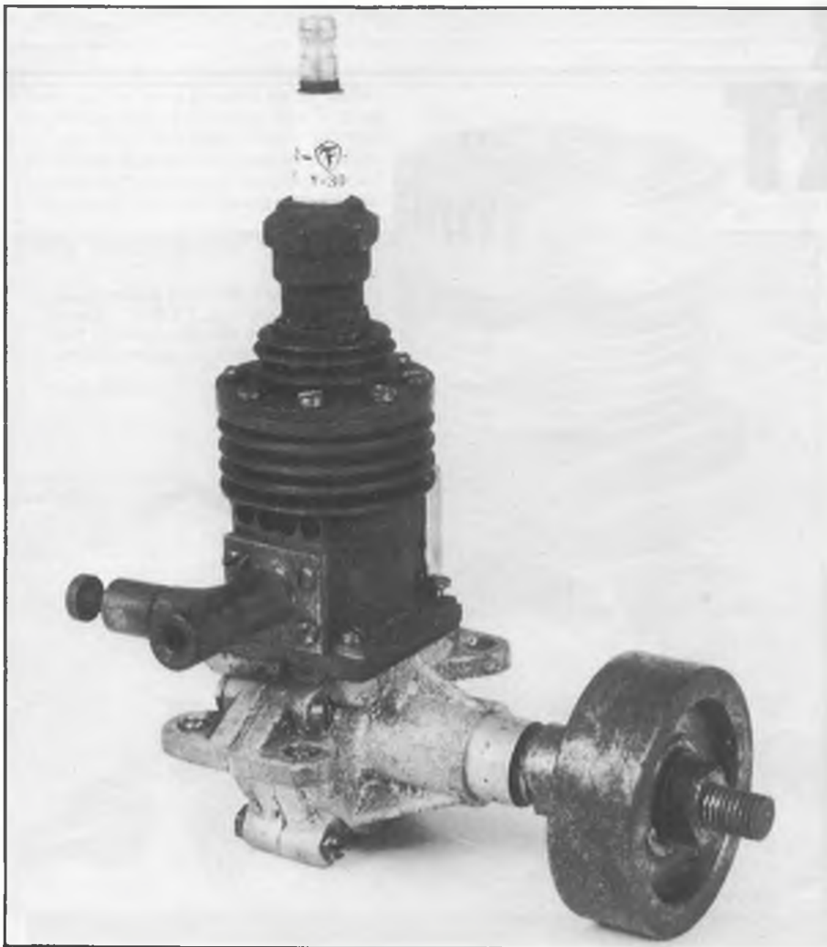
Above: Instantly recognisable - a kit-built GHQ, at least forty years old. Fitted for flywheel operation and crowned with full-size spark plug, this remarkable but incomplete specimen contrasts with (below) a newly discovered Loutrel - the fuel tank is genuine vintage fitting! - and an airworthy GHQ. See text...
