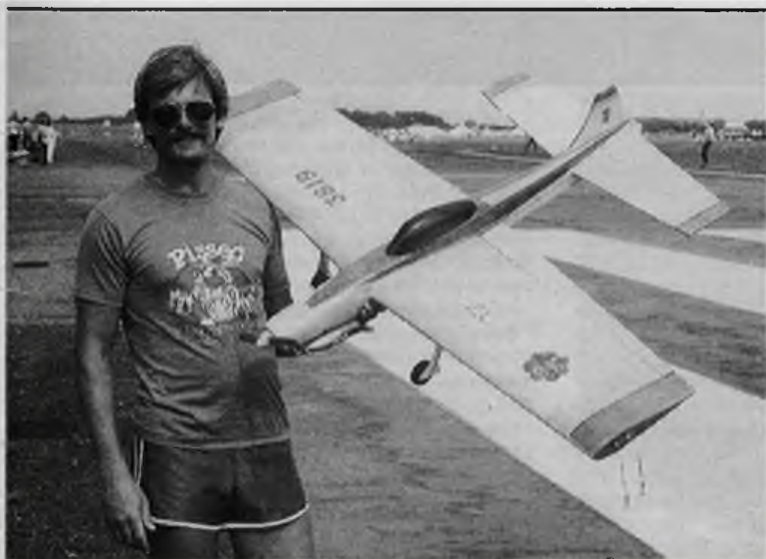
Above: Unusual Russian combat wing features nylon or mylar covering, 'tensioned-bow' leading edge and wire T.E. Anyone care to try it?
