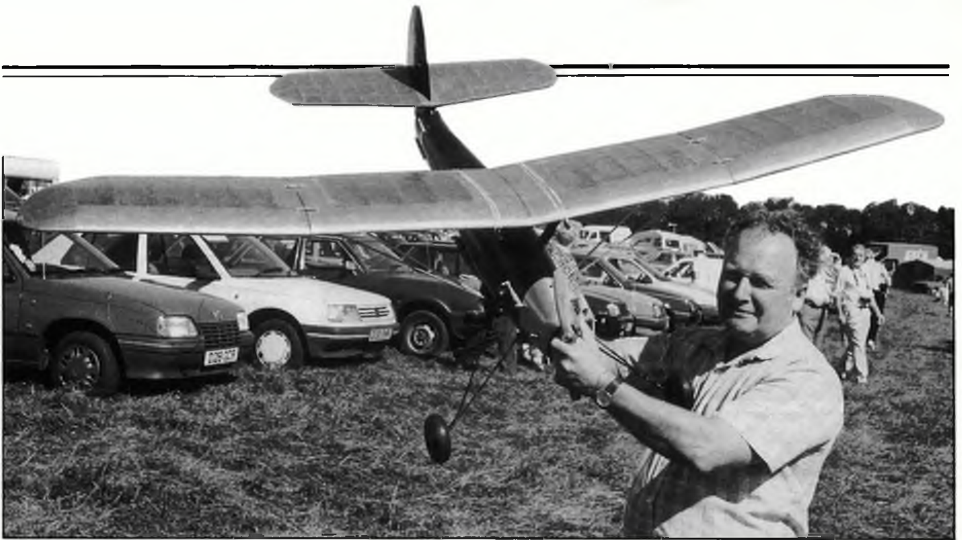
Above: Described in Vintage Extravaganza last November was Charlie Havis' 1946 Bowden Trophy Winner, a design by Alec Wilson of Hayes that dismantles into quite a small package thanks to hooks and rubber bands at the tail unit and outer wing panels.
