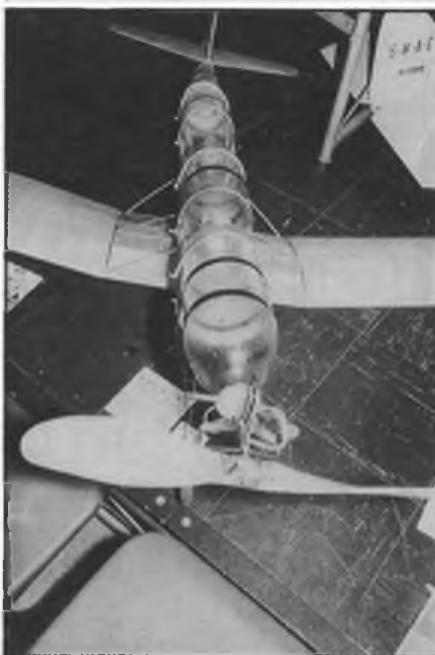
Above: Jack Humphreys showed a Joe Ott compressed air monoplane - modified to take three coupled Tizer plastic bottles - at Shefford in October 1982 when SAM 35 held their first National Exhibition. Note use of a folding propeller, for reasons mentioned in text.
