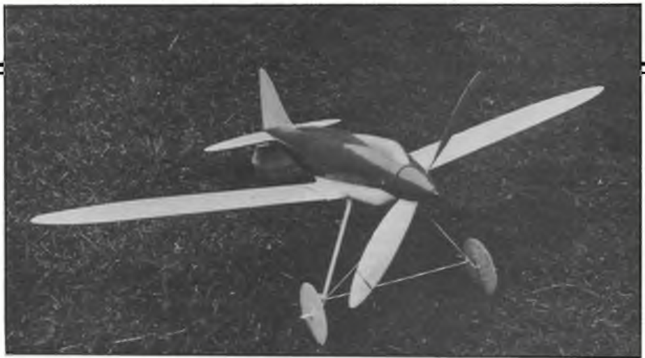
Above: A three-cylinder Pavely engine and miniature container were used by James Pelly-Fry in his sleek 1931 racer (wing loading was fourteen ounces per square foot!) which was designed to attack the SMAE speed record of 32 mph, over 100 yards, then held by R.N. Bullock.
