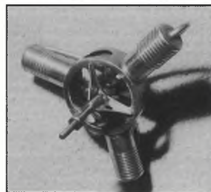
This three-cylinder F J Camm engine, described in various early publications, was made by Jack Humphreys. An identical was used by Tony Turner in the model at top of page.
