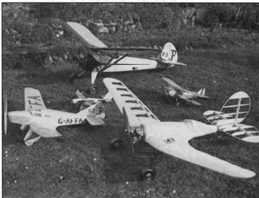
Right: Prototype Porlock Puffin on its home field. Powered by the 2.3cc Spitfire engine it was the result of a combined effort by CEB and Doctor Forster to produce a powered glider that would actually climb on the very low amount of power available.
