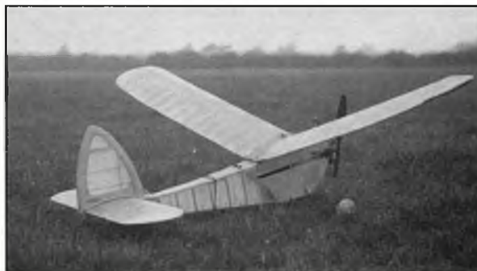
Right: Prototype Porlock Puffin on its home field. Powered by the 2.3cc Spitfire engine it was the result of a combined effort by CEB and Doctor Forster to produce a powered glider that would actually climb on the very low amount of power available.
