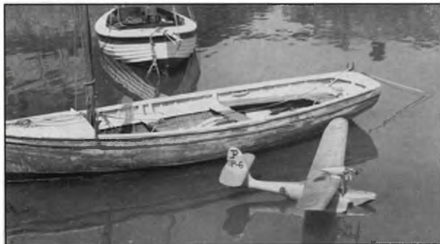
Above: Cabin version of P-3 made in November 1939 reverted to the original size of the Moyer Cloud Cruiser. Baby Cyclone fitted to a Bowden detachable elektron mount sports an early attempt to cowl the engine using a Grip-Fix tin. Left: Never attracted to control-line when it later came to this country, Doctor Forster did try some tethered flying. He is seen here playing the cabin P-3 on his trout fly rod and line around Christmas 1939.
