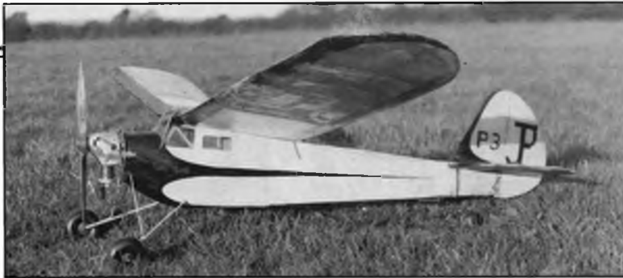
Above: Cabin version of P-3 made in November 1939 reverted to the original size of the Moyer Cloud Cruiser. Baby Cyclone fitted to a Bowden detachable elektron mount sports an early attempt to cowl the engine using a Grip-Fix tin. Left: Never attracted to control-line when it later came to this country, Doctor Forster did try some tethered flying. He is seen here playing the cabin P-3 on his trout fly rod and line around Christmas 1939.
