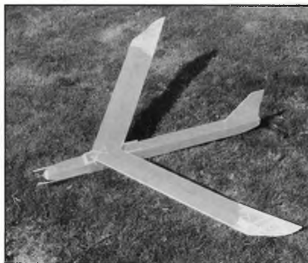
Above: Construction is straightforward, even if the wing is a bit unusual by modern standards. Left: Pipistrelle's lines are austere but attractive. Long fuselage means plenty of room for rubber. Below: Plenty of scope for longitudinal wing adjustment.
