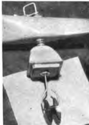
Fig. 10, left : The bobbin is slipped onto the end, and the shaft bent round as shown. Since the bobbin is a very loose fit on the wire, it must be packed tightly in place by means of a wedge of hardwood.
