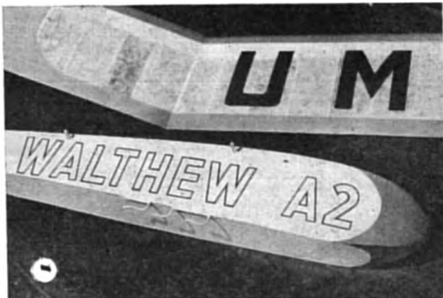
Fig. 7. Below, left, ready for assembly. Borders and nose finished in bright red, letters and pennant in dark blue. Fig. 8. Below, right, the other side of the fuselage, showing 2" transfer letters and 4" cut out tissue letters applied to the wing with clear dope.
