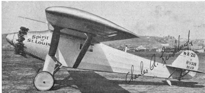
Just made! At San Diego, the original Spirit of St. Louis awaits its axle covers, carb heater and the few hours of flying experience prior to its 33 1/2 hour crossing of the Atlantic. Span 46 ft. Length 27 ft. 8 in. Height 9 ft. 10 in. Chord 7 ft. Incidence 0 degrees. Weight for normal flight 1,700 lb. Weight at take-off 5,250 lb. Ultimate range, 4,110 miles (Erickson photo)
