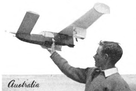
Max Effe with his canard flying boat "Puddleduck", designed by Jim Fullarton. Note floats under wings and stepped hull
