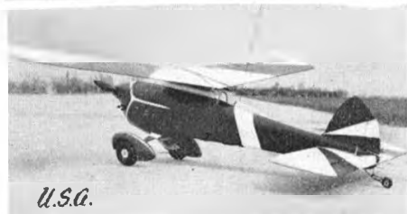
Lars Gunnar Larsson was winner of winter contest for rubber models in SWEDEN. Nifty colour scheme in red and white is on a pylon wing R/C model by Capt. Mike McGuinn of Fort Eustis, Virginia, U.S.A. Wing is from a Sterling "Mamba" kit, has rudder, elevator and motor control. Citizenship receiver. Babcock escapements
