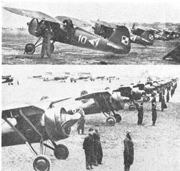
PZL P-11 fighters of 113 Squadron warming up their engines at Warsaw Okęcie airport. Closest to the camera is a four gun P-11c, with two P-11a behind it and then more P-11c's. Line up below shows the purposeful, if outdated lines of the aggressive P-11, surely a fine modelling subject for flying scale?
