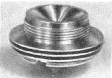
Cox Tee Dee 15 breaks 16,000 on an 8x4! Close-up reveals the bell section head contour and view below shows black plastic carburettor housing. British supplies expected soon!
