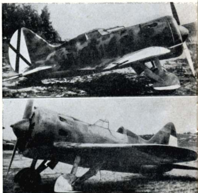
Upper picture shows the sliding cockpit canopy in aft position on Republican Air Force I-16 type 6, aircraft IW-1. Below is a type 10 aircraft in Nationalist markings, showing the fuselage mounted guns and fixed windshield without cockpit cover
