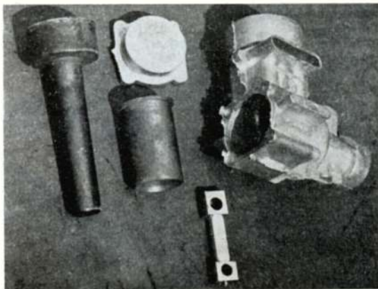
Left, a Super Tigre G.20 V in the raw. Die-cast crankcase and rear cover, forged crankshaft and rough machine cylinder liner and connecting rod. Right, well known Italian speed flyer Amato Prati at the assembly bench with deft experienced fingers which go to maintain a renowned Italian standard of workmanship
