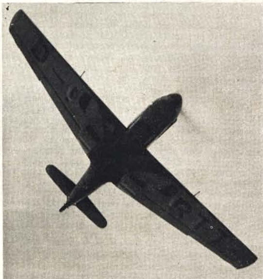
Above right, factory photograph with “Swastika” deleted shows a preserved 109E AJ-YH with splinter camouflage and dappled sides, note early hood. Above, Bf 109V14 (D-1RTT), first prototype of the E series with DB601A engine, two fuselage guns and two wing cannons, first flown in summer 1938. Note unusual colour line under centre. (Messerschmitt A.G. photo.)
