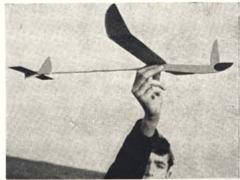
Tailplane cemented to boom
