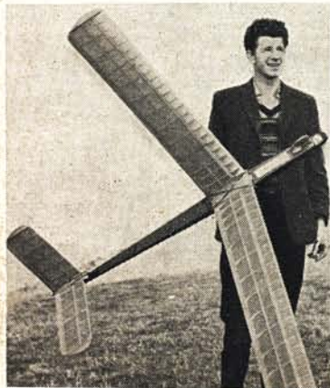
St. Albans Free Flight soaring aces at last year's Luton organised slope contest. Left, winner Don Edwards, with 70 in. pendulum Nose Vane "Super Woggis" design which weighs only 22 oz. and takes 22 hours' building time! Below, is Colin Morris with 34 in. all-sheet "Woggis". Note use of forward fin.
