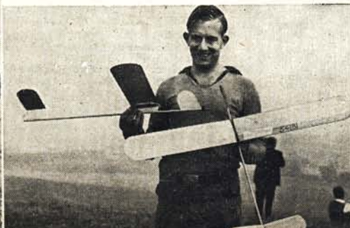
St. Albans Free Flight soaring aces at last year's Luton organised slope contest. Left, winner Don Edwards, with 70 in. pendulum Nose Vane "Super Woggis" design which weighs only 22 oz. and takes 22 hours' building time! Below, is Colin Morris with 34 in. all-sheet "Woggis". Note use of forward fin.
