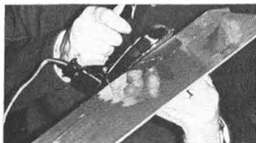
Using domestic iron set at "wool", heat seal all wraps with gentle rolling action, start at centre, working to ends.
