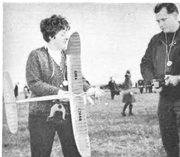
Shirley and Bill Horton of Crawley winding the rubber motor of Roger Schroeder's (U.S.A.) Coupe d'Hiver model at Chavenay, France. Note the use of drill winder with trip odometer to indicate number of turns.
