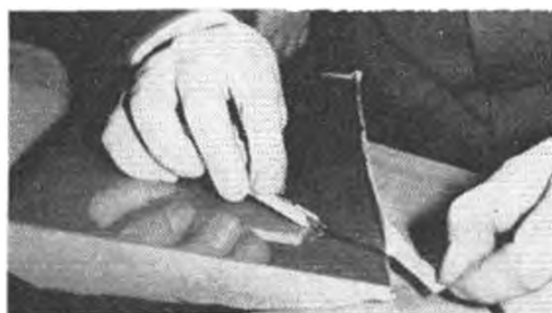
Set iron to "rayon" and glide over the MonoKote. It heat shrinks quickly. Move iron to fresh area as colour change appears, wrinkles disappear and colour resumes original high gloss as reflection of Max Coote's face indicates at right.
