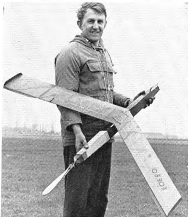
Tail-less winner at Tern Hill was Ken Attiwell with pusher that employs rearward folding prop and side-lifting nose fin for stability.
