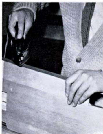
Sealing the edge is accomplished by 'rolling' the iron over the trimmed overlap edge of the film. Use a light-weight travelling iron to avoid building up extra arm muscles on one side only and be careful not to melt the film with prolonged contact.
