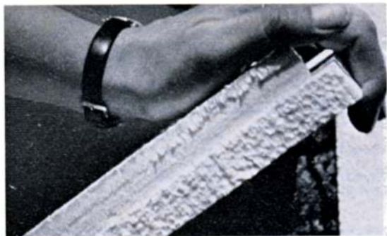
Figure 3 above, illustrating a clean cut by knife in the upper panel, lower panel has natural edge finish.
