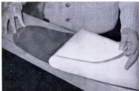
Peeling the paper backing piece from the panel. Some modellers prefer to do this in stages as the panel is adhered to the framework. Our preference is to take all the paper off.
