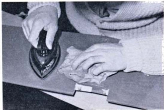
The iron is set for 'Rayon' or 'Wool' and held over the film to transfer heat and so shrink the film taut over the wing. Blisters and wrinkles disappear and the final touch of the iron on the surface (lightly mind!) sets the heat sensitive adhesive on the sheet surfaces.
