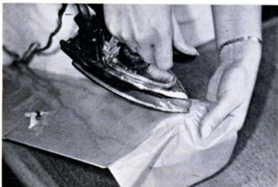
Working around a compound curve of a wingtip demands a little patience. It is surprising how the film will adopt two-way curves though sometimes it is necessary to cut and overlap strips on sharply-curved tips.
