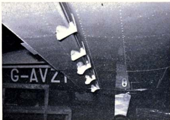
Slotted flaps and ailerons have protruding hinge plates. Note the tab in starboard aileron only, picketing ring and streamline undercarriage fairing.
