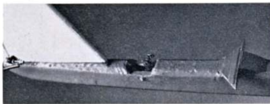
Rigid fin construction and positive tailplane mounting are essential features of this extremely well-developed contest design which has variable incidence tailplane (V.I.T.), auto-rudder (A.R.) and dethermaliser (D/T) controls from a Hans Seelig timer in the fuselage.
