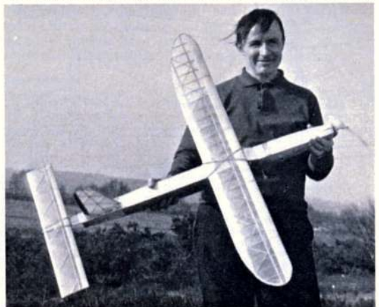
Left, Ian Kaynes with his tailless rubber model. Note tips joined to inner panels via sheet fins. Right, Bill Houghton displays his remarkable 'Melinex' covered rubber model. See also page 302.
