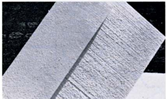
Figure 5 above shows a panel which has sanded surface compared with cut surface of raw block as supplied. Below is Figure 6 which illustrates how waste areas are marked and templates pinned in place.
