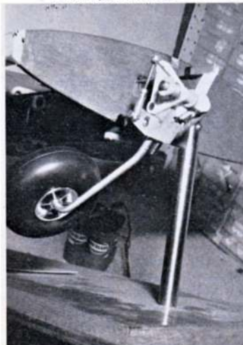
Above: amazingly positive and effective retracting undercarriage unit by Micro-Mold Accessories is servo-operated. Below right: Micro-Mold also do cockpit canopy and top deck for Aeromodeller Oct. 1968 Beagle Pup.
