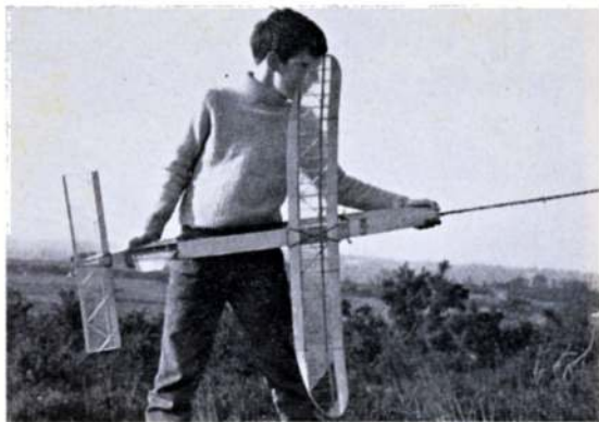
Transparent Melinex covering on this contest model by Bill Houghton does not exactly aid visibility though sun reflection from the exceptionally smooth surface is considerable. See a glider tail at right, with rigid structure to preserve shape.
