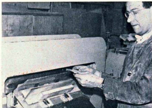
The 'Slicing' machine which produces contoured sheet balsa wings for ready-to-fly models from a block. The operator is holding three wings.
