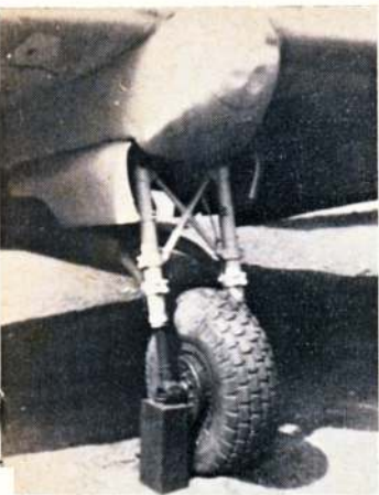
Close-up of starboard undercarriage assembly of IL-2 m3 at Polish Armed Forces Museum in Warsaw. Tyre tread pattern is not typical of wartime Soviet machines. Note the almost flat sides of the streamlined container.
