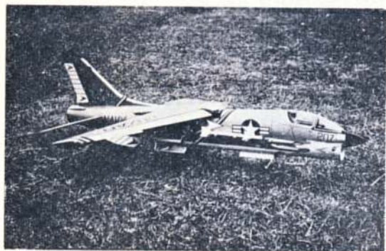
Left, Maurice Mitchell's magnificent Crusader , which took third place in the control-scale event, featured variable incidence wing, controlled in flight, plus arrester hook, retracting undercarriage and both leading and trailing edge flaps.
