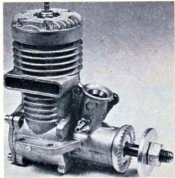
1961 Fox 40. 1962 crankcase had wider mounting lugs and was also used for later Rocket 35's.
