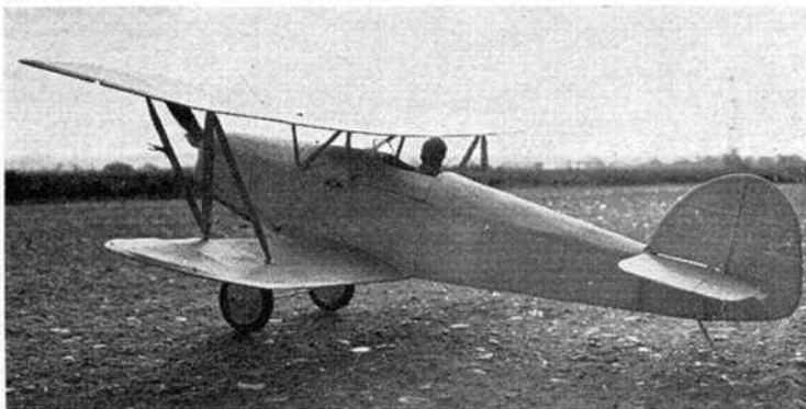
Andrew Callaghan's Isaac's Fury could be taken for a 'proper' free flight scale model (if not the real thing!) but who would believe that it is only 14 in. span! Flies extremely well too - in fact it is becoming quite a veteran now. Plenty of wing area and low weight contribute towards this, together with careful trimming of course . . .
