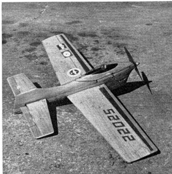
First of Jim Broad's current series of F.A.I. racers, based on Russian Plotsin/Timofeev model. Tissue covered, the model weighs just 16½ oz. with its HP15D powerplant, despite repair jobs which indicate its hard life!
