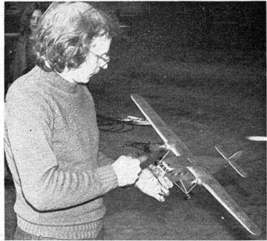
Andrew Callaghan 'runs-up' the motors of his Avro 642. Power is supplied by single skein motor consisting of four strands of 1/4 in. flat rubber in the fuselage, driving a step-up gearbox in the nose. Power is then transmitted back to the centre via a flexible shaft and outboard to the two prop shafts! Let's hope that the friction involved does not lose too much efficiency.
