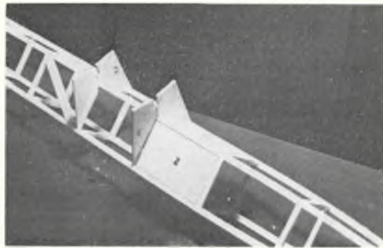
The Mentor's fuselage is basically a square box which is then tilted onto one corner to form a diamond shape.
