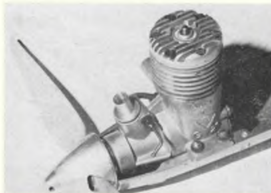
Rod Brown's Super Tigre 29FI - note the \frac{1}{8} in. venturi and Rossi needle in ST spraybar. Has ABC piston/liner (pipe timed) and experimental Cox 15 insert-type head. Twice previous holder of NZ record, now being prepared for new attempt.
