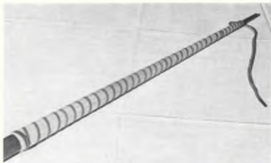
At left the fuselage boom is being laminated - two layers of 0.8mm balsa are bound to the mandrel whilst drying out. See text for details.
