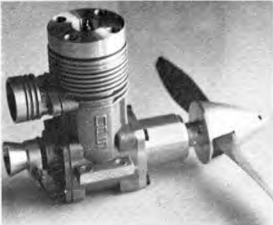
Andy Keiller's much modified OPS 60 which uses many Super Tigro parts as well as home-made front housing. Already bettered 204mph, with promise of more to come. See text for details.
