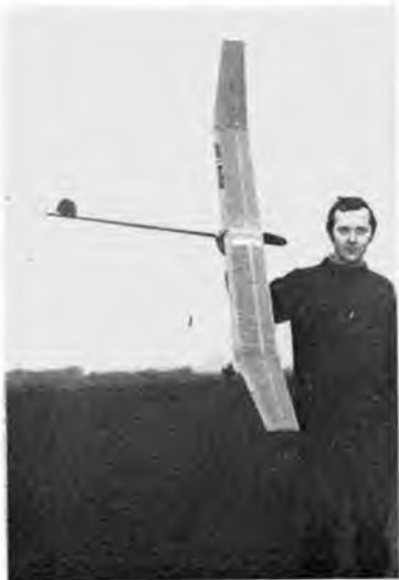
Mike Woodhouse and his approach to tapered tips – his new A/2 features Benedek 6354/b airfoil, Maxaid circle towhook, and is called 'Whiffler'.
