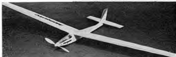
KATY A2 SAILPLANE ... £15.80 Span 67". A true contest model with auto-rudder and dethermaller.
