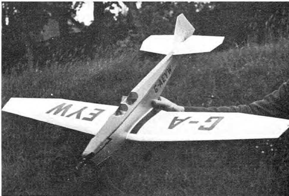
Original FIF Scale model by John Coasby powered by D.C. Dart inside sheet engine cowling of Citrus Minor version.
