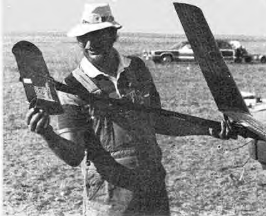
Above: Bill Gieskieng with his latest FAI folder, attending to the folding fin! Left: Timer mechanism set for climb with wings folded and parallelogram pylon skewed forward.
