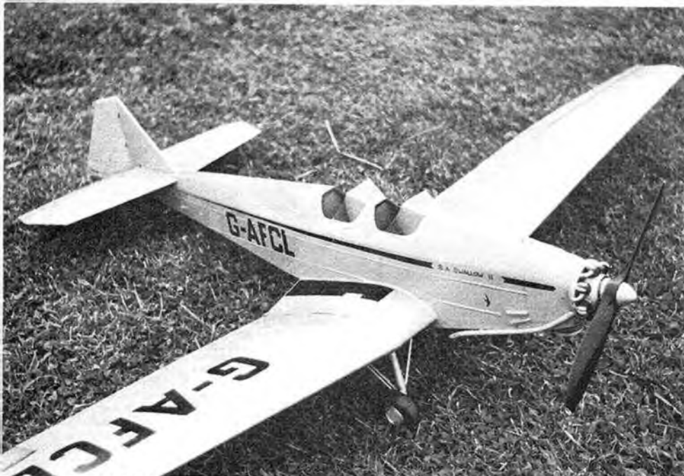
Superb CIL Scale model by Colin Essex, with inverted PAW 19 motor concealed inside dummy Pobjoy engine.
