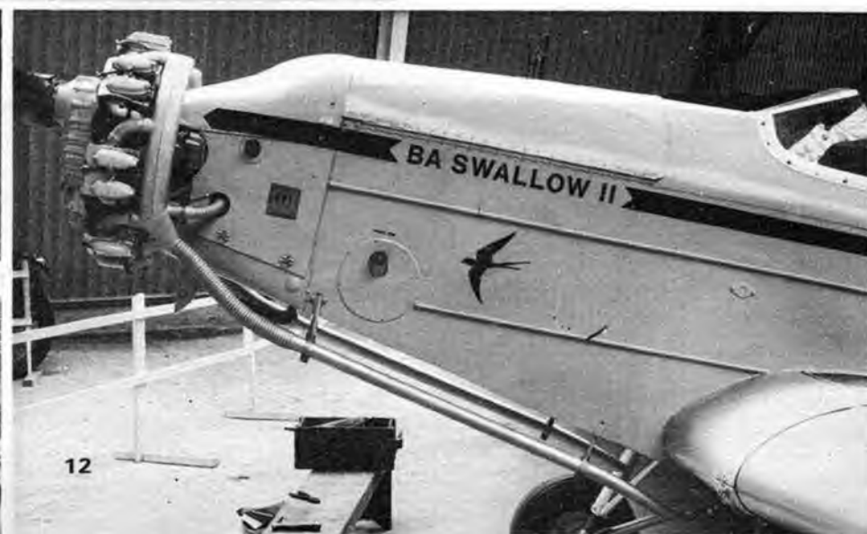
7. Petrol filler cap and compass set in port wing alongside wing root walkways. 8. Telescopic undercarriage leg and supporting struts. Note brake pipe to wheel hub and clip to thin ply wing joint cover strip. 9. Venturi to airspeed indicator on starboard side. Instrument panels; front passenger cockpit 10 ; and rear pilot's cockpit. 11. 12. Port side view shows metal nose cowling to Pobjoy engine, note Mandarin Hotel sticker.
