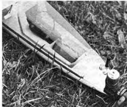
Power pod nose on Edmonds Model Products Cock Sparrow shown fitted with Testor 049. Small motor allows gradual height gain from extended motor run prior to glide.
