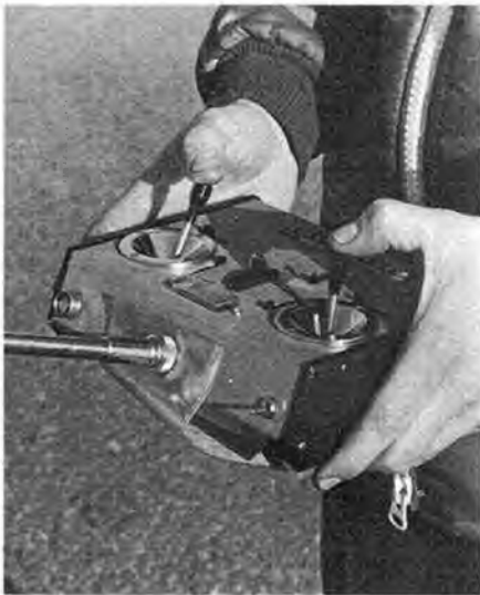
How to hold the transmitter is largely a matter of personal choice. Left "Thumbs" method allows transmitter to be gripped firmly in hands; right "Finger and Thumb" grip may offer greater control but really needs neck strap to support transmitter.
