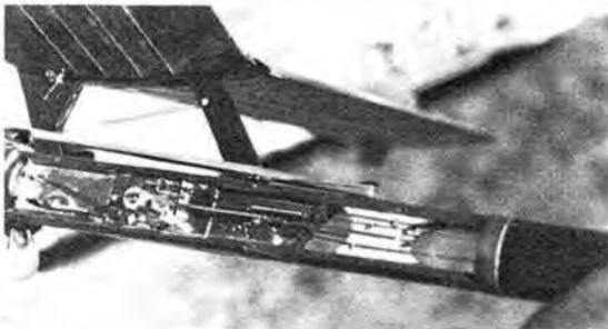
Above: Bill Gieskieng with his latest FAI folder, attending to the folding fin! Left: Timer mechanism set for climb with wings folded and parallelogram pylon skewed forward.
