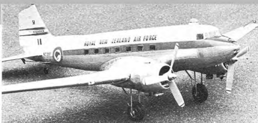
Control Line Scale DC3 powered by two OS 10s, by Stan Rusbatch of the Oamaru Power Model Aero Club of New Zealand. A most impressive model which is covered with aluminum foil on wings, tailplane and lower fuselage, complete with simulated 'rivets'. Lights operate and cowls are made from plastic bottles.
